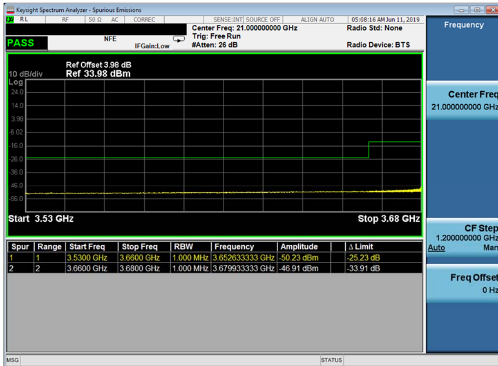
Plot 7-28. Conducted Spurious Plot (Band 48 - 20.0MHz QPSK - RB Size 1, RB Offset 99 - High Channel)
