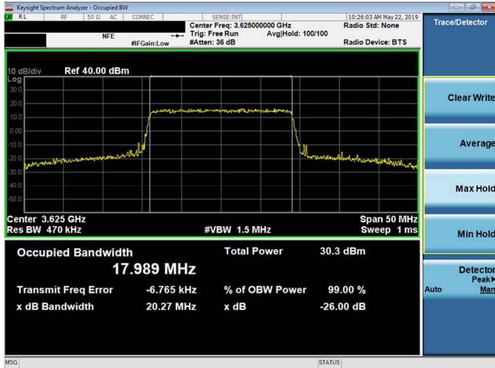
Plot 7-13. Occupied Bandwidth Plot (Band 48 - 20.0MHz QPSK - Full RB Configuration)
