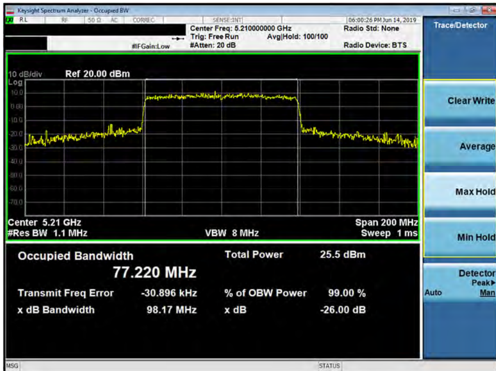
Plot 7-69. 26dB Bandwidth Plot SISO ANT2 (80MHz BW 802.11ax – Full Tones (UNII Band 1) – Ch. 42)
