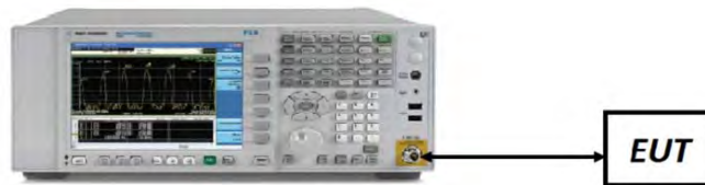
Figure 7-2. Test Instrument & Measurement Setup
