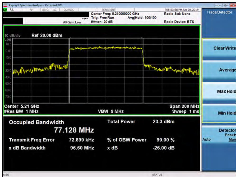
Plot 7-27. 26dB Bandwidth Plot SISO ANT1 (80MHz BW 802.11ax – Full Tones (UNII Band 1) – Ch. 42)
