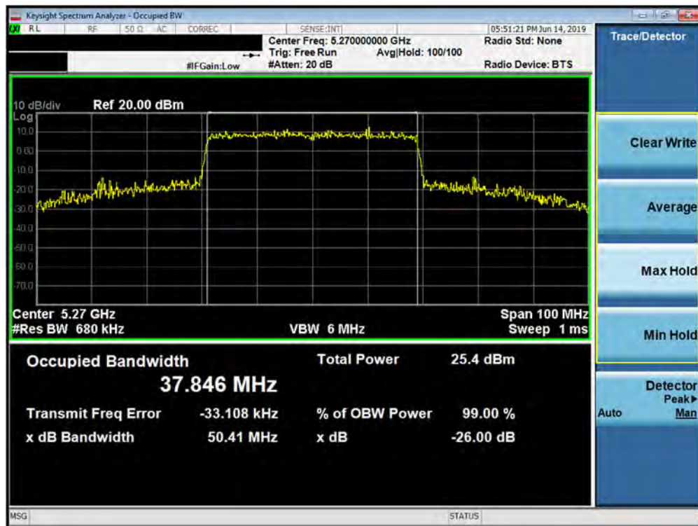
Plot 7-73. 26dB Bandwidth Plot SISO ANT2 (40MHz BW 802.11ax – Full Tones (UNII Band 2A) – Ch. 54)
