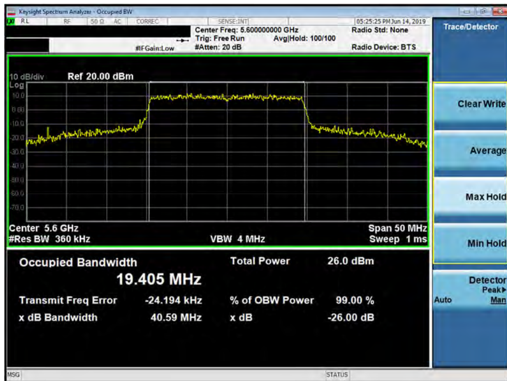
Plot 7-77. 26dB Bandwidth Plot SISO ANT2 (20MHz BW 802.11ax – Full Tones (UNII Band 2C) – Ch. 120)
