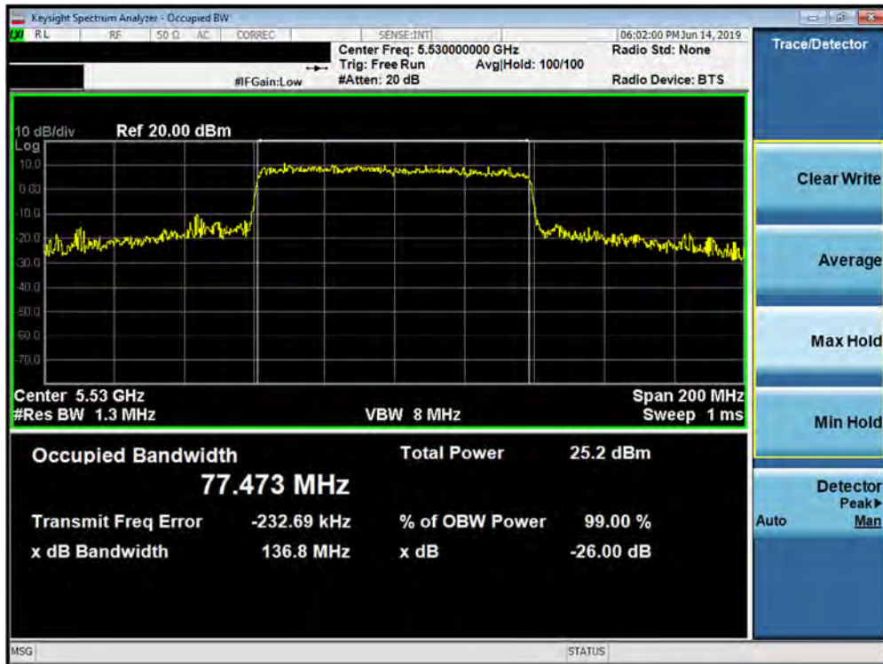
Plot 7-82. 26dB Bandwidth Plot SISO ANT2 (80MHz BW 802.11ax – Full Tones (UNII Band 2C) – Ch. 106)
