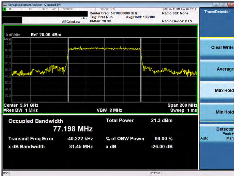
Plot 7-41. 26dB Bandwidth Plot SISO ANT1 (80MHz BW 802.11ax – Full Tones (UNII Band 2C) – Ch. 122)
