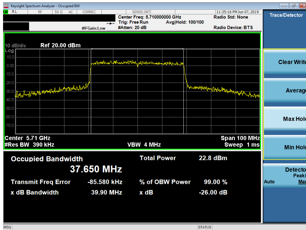
Plot 7-96. 26dB Bandwidth Plot SISO ANT2 (40MHz BW 802.11ax (UNII Band 2C) – Ch. 142)
