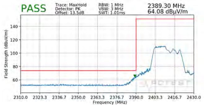
Plot 7-124. Radiated Restricted Lower Band Edge Measurement MIMO (Peak – 106 Tones)
