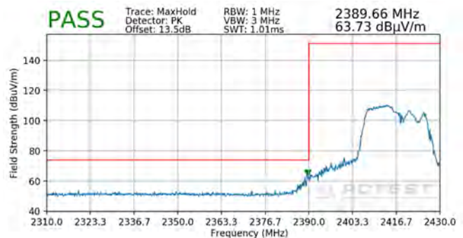
Plot 7-126. Radiated Restricted Lower Band Edge Measurement MIMO (Peak – 106 Tones)
