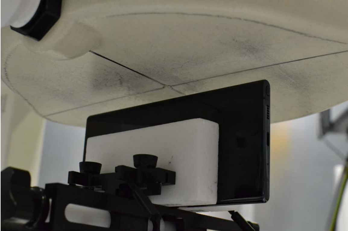
SAR Test Setup Photo 17 – Right Side at 10 mm
