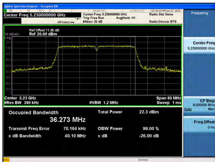
802.11ac_VHT40 UNII 2C BAND 26dB Bandwidth(CH 118)
