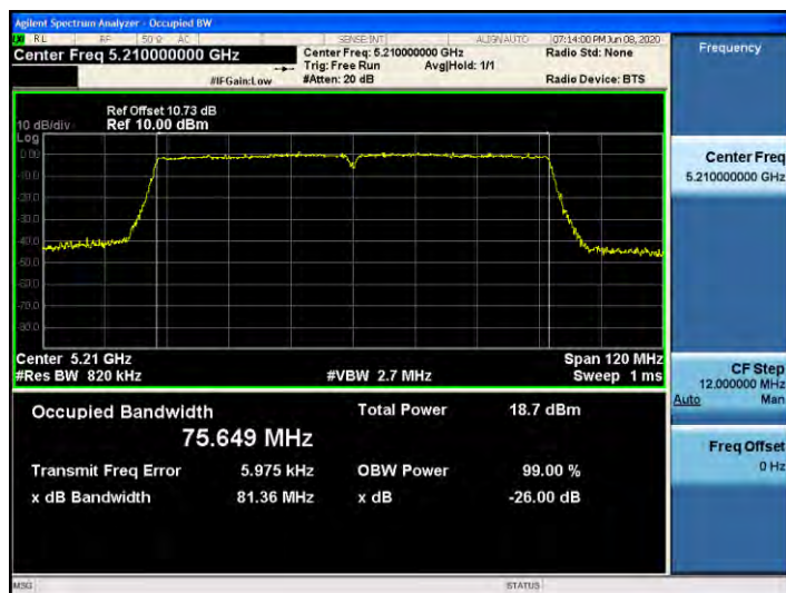
802.11ac_VHT80 UNII 2C BAND 26dB Bandwidth(CH 138)
