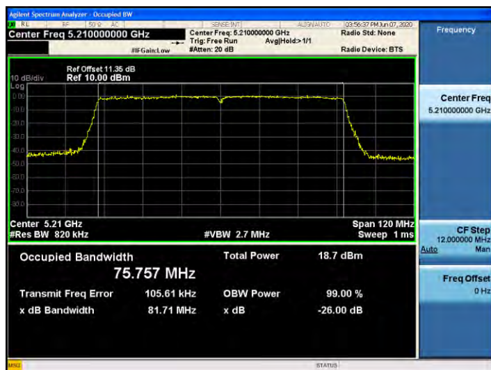
802.11ac_VHT80 UNII 2C BAND 26dB Bandwidth(CH 122)
