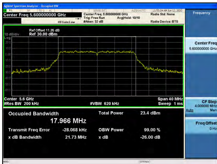
802.11ac_VHT20 UNII 2C BAND 26dB Bandwidth(CH 120)
