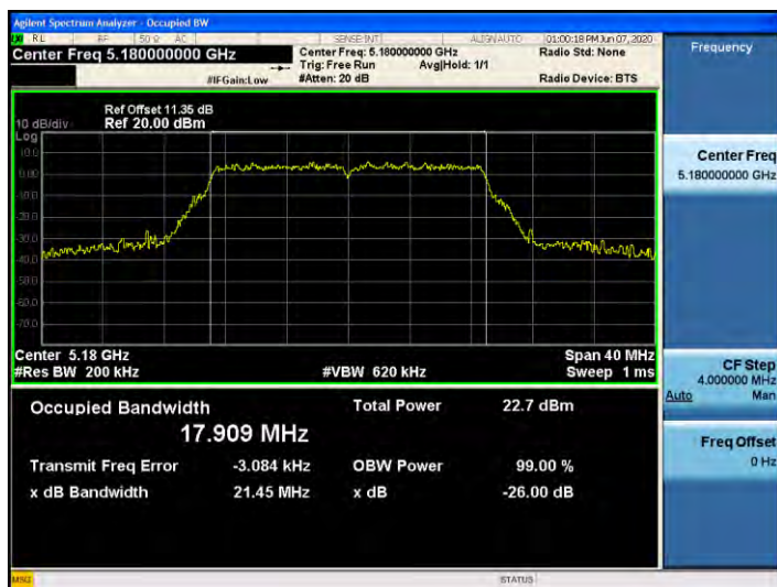
802.11ac_VHT20 UNII 2C BAND 26dB Bandwidth(CH 120)
