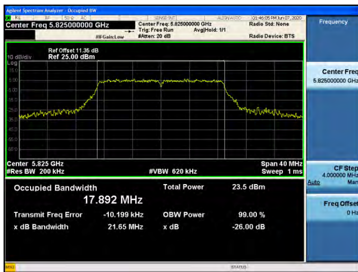
802.11ac_VHT20 UNII 3 BAND 26dB Bandwidth(CH 165)
