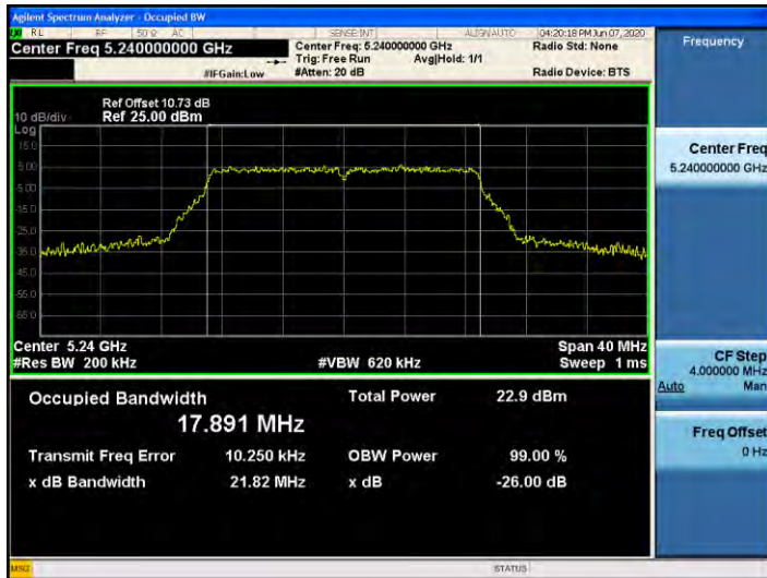
802.11n_HT20 UNII 2C BAND 26dB Bandwidth(CH 144)
