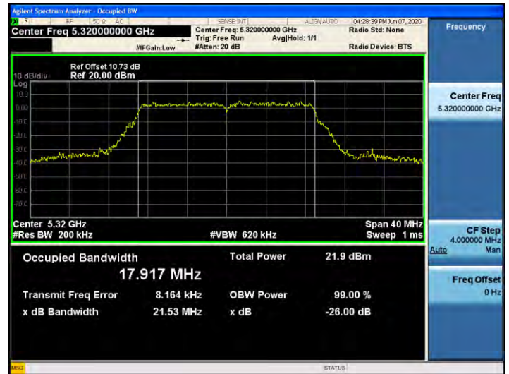
802.11n_HT20 UNII 3 BAND 26dB Bandwidth(CH 165)
