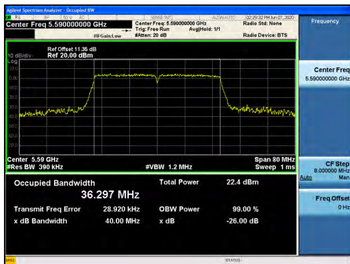
802.11ac_VHT40 UNII 2C BAND 26dB Bandwidth(CH 118)
