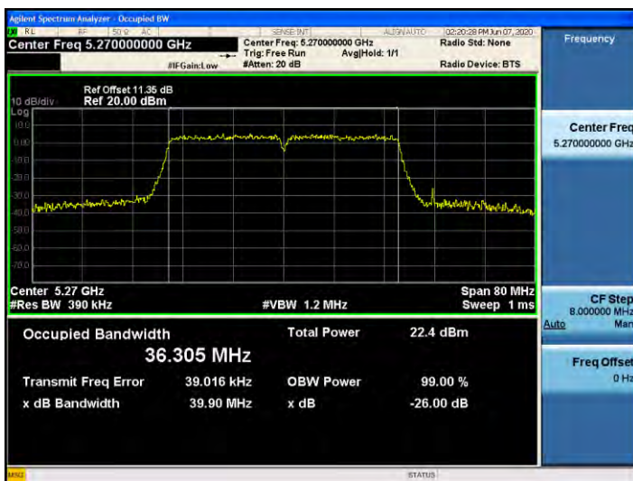
802.11ac_VHT40 UNII 3 BAND 26dB Bandwidth (CH 159)
