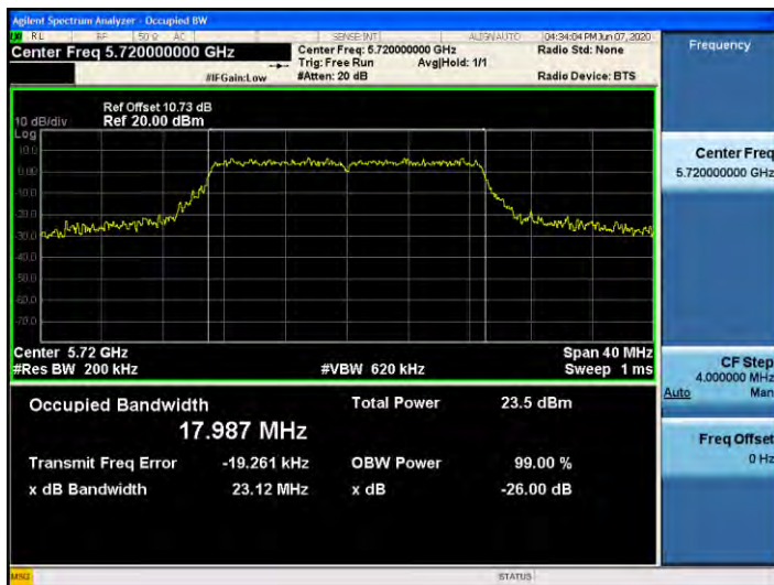
802.11n_HT20 UNII 2C BAND 26dB Bandwidth(CH 144)
