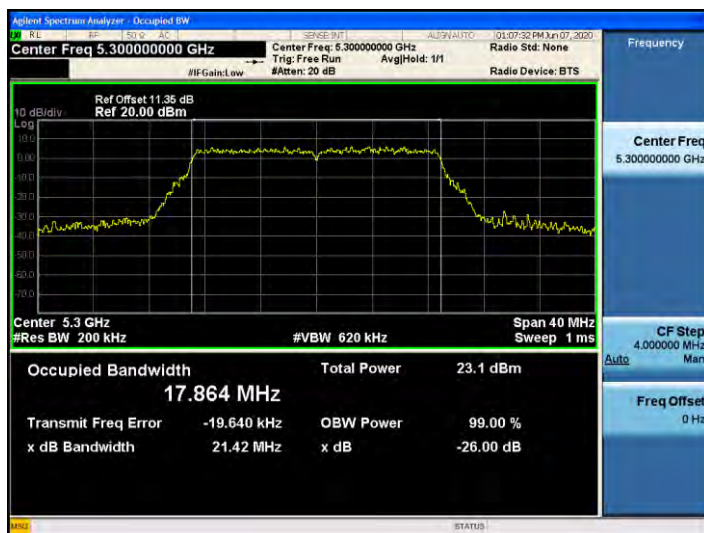
802.11ac_VHT20 UNII 3 BAND 26dB Bandwidth(CH 165)
