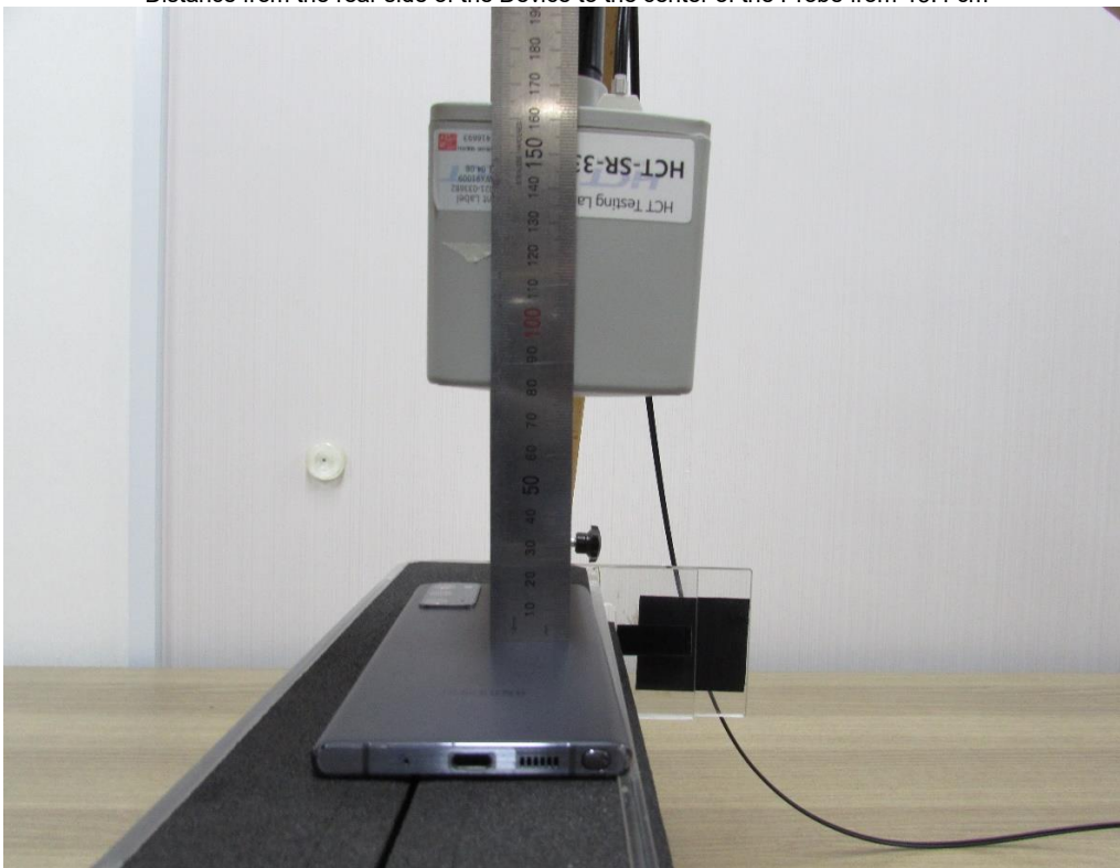
Distance from the rear side of the Device to the center of the Probe from 13.4 cm
