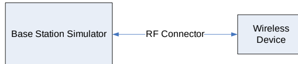
Figure 9-4 Power Measurement Setup
