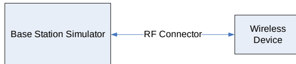
Figure 9-2 Power Measurement Setup
