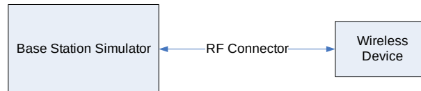
Figure 9-1 Power Measurement Setup
