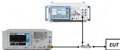
Figure 7-3. Test Instrument & Measurement Setup
