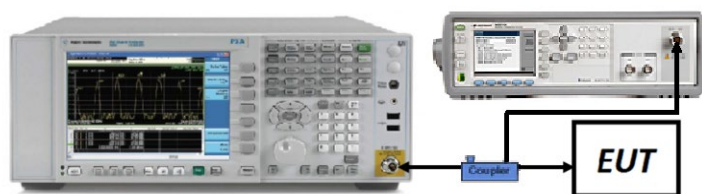
Figure 7-3. Test Instrument & Measurement Setup
