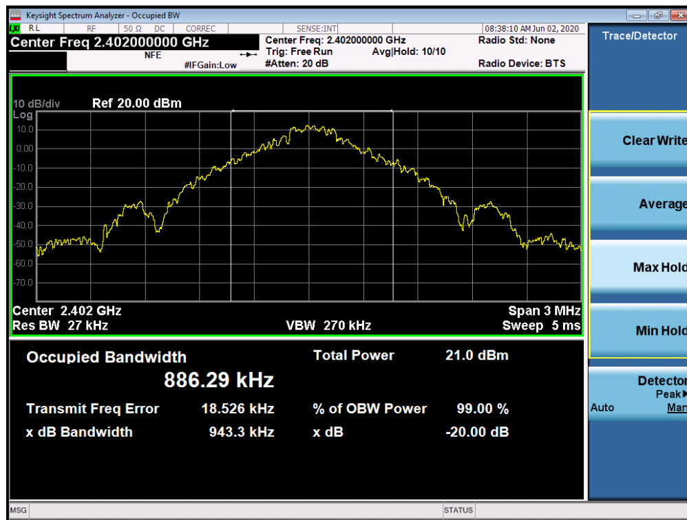
Plot 7-1. 20dB Bandwidth Plot (Bluetooth, 1Mbps – Ch. 0)
