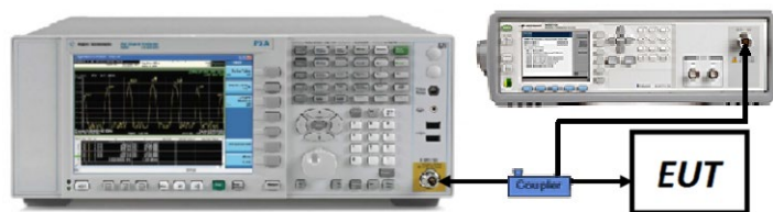
Figure 7-7. Test Instrument & Measurement Setup
