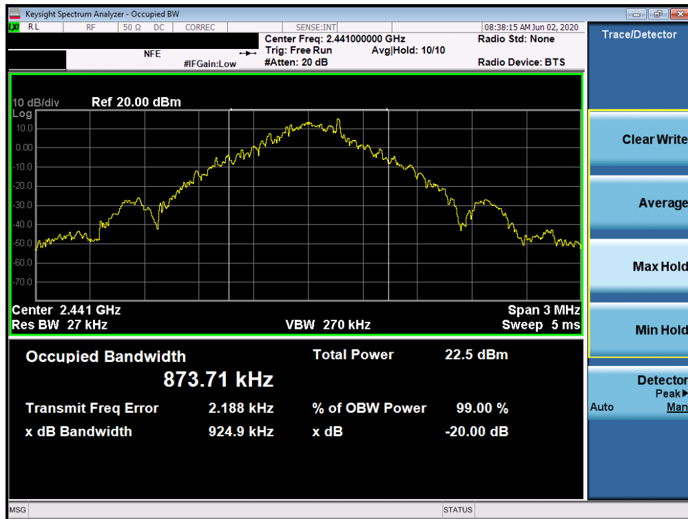
Plot 7-2. 20dB Bandwidth Plot (Bluetooth, 1Mbps – Ch. 39)
