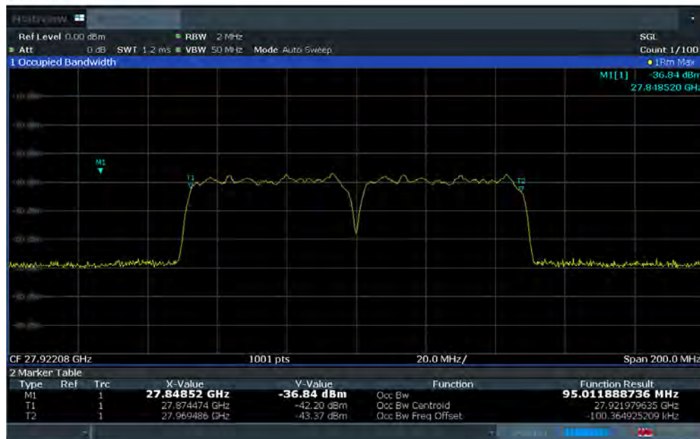
Plot 7-8. Ant 1 Occupied Bandwidth Plot (50MHz-2CC – pi/2-BPSK – Mid Channel)
