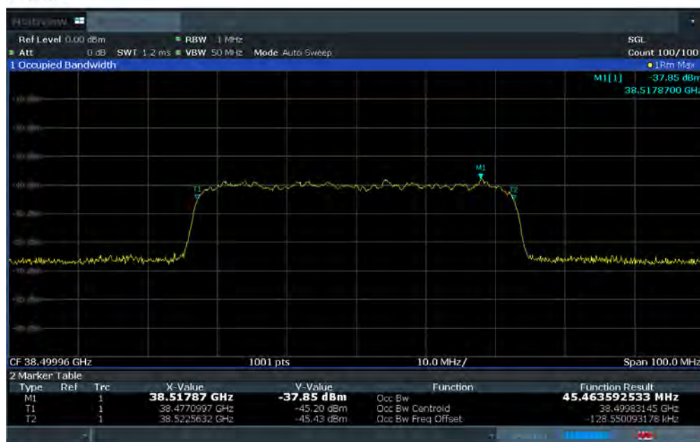
Plot 7-20. Ant 1 Occupied Bandwidth Plot (50MHz-1CC – pi/2-BPSK – Mid Channel)
