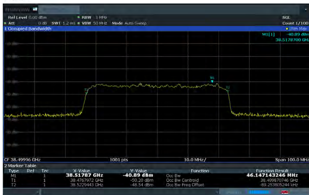
Plot 7-18. Ant 1 Occupied Bandwidth Plot (50MHz-1CC – 16QAM – Mid Channel)
