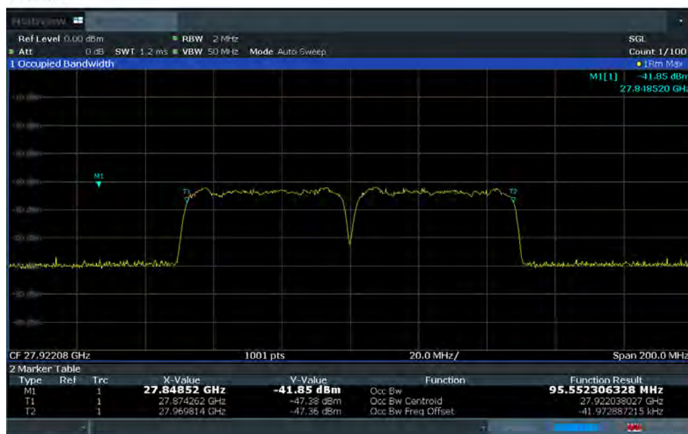
Plot 7-6. Ant 1 Occupied Bandwidth Plot (50MHz-2CC – 16QAM – Mid Channel)
