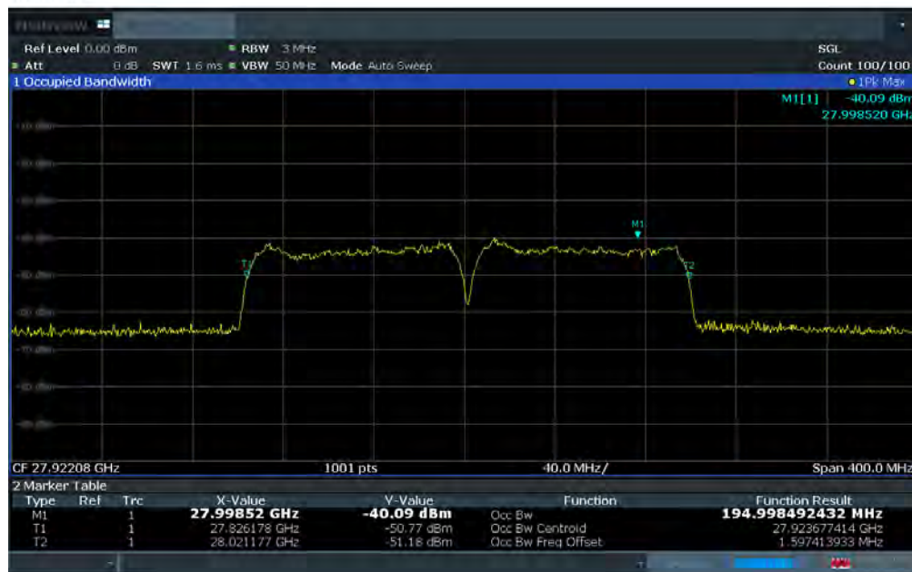
Plot 7-15. Ant 1 Occupied Bandwidth Plot (100MHz-2CC – 64QAM – Mid Channel)
