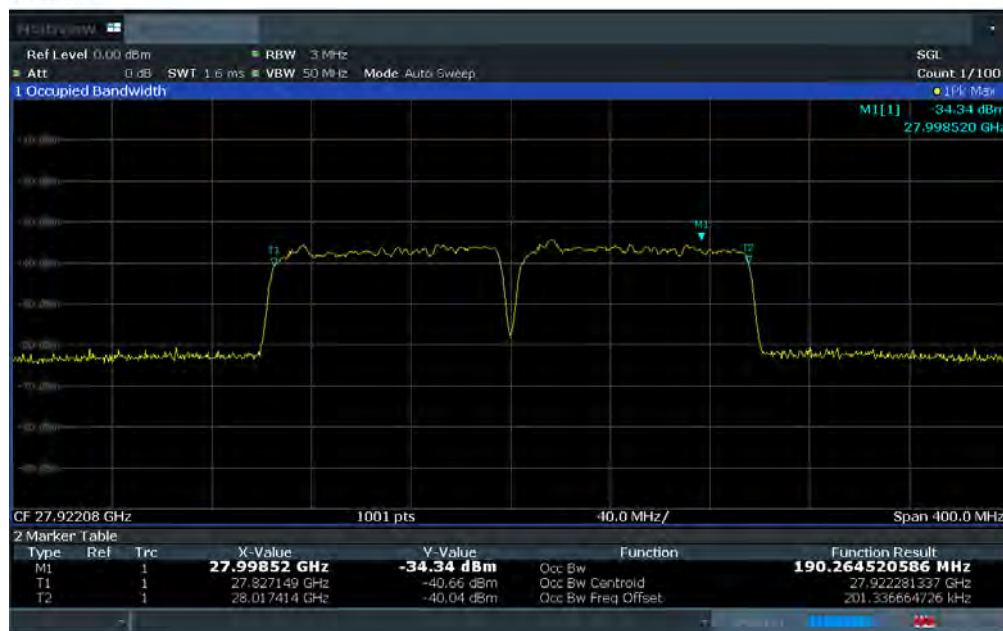
Plot 7-16. Ant 1 Occupied Bandwidth Plot (100MHz-2CC – pi/2-BPSK – Mid Channel)
