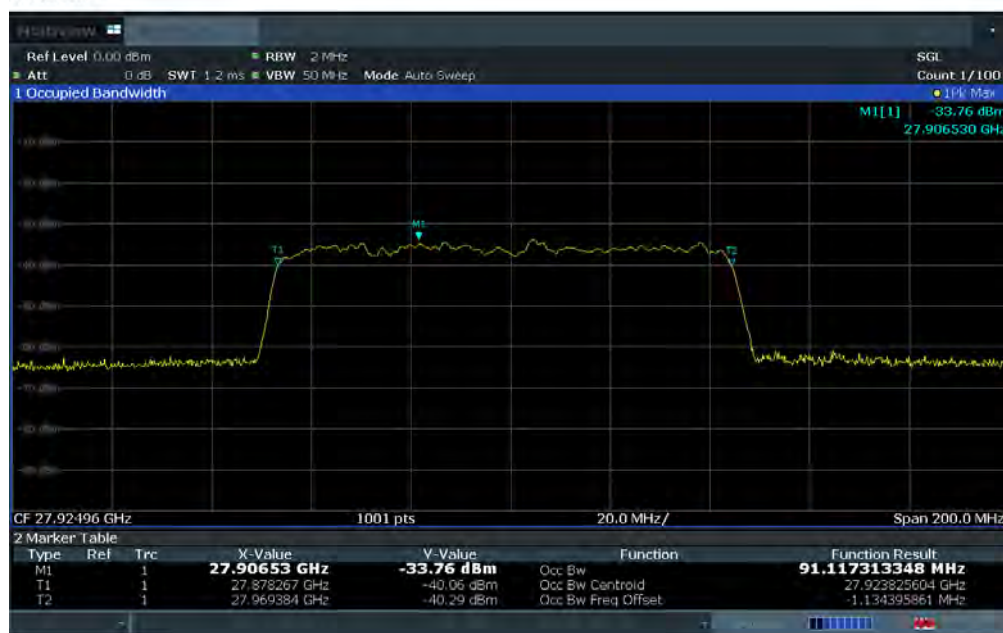
Plot 7-10. Ant 1 Occupied Bandwidth Plot (100MHz-1CC – 16QAM – Mid Channel)
