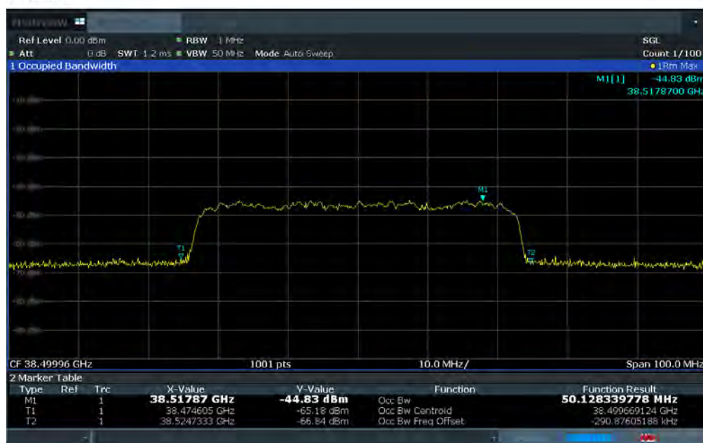
Plot 7-19. Ant 1 Occupied Bandwidth Plot (50MHz-1CC – 64QAM – Mid Channel)
