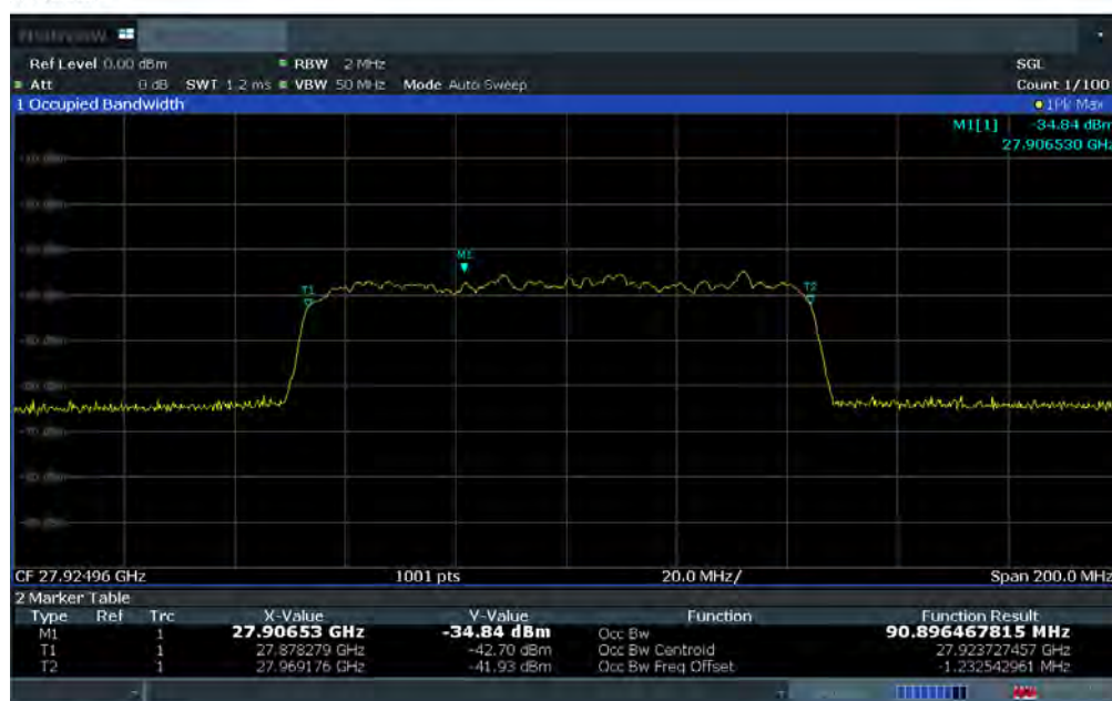
Plot 7-11. Ant 1 Occupied Bandwidth Plot (100MHz-1CC – 64QAM – Mid Channel)
