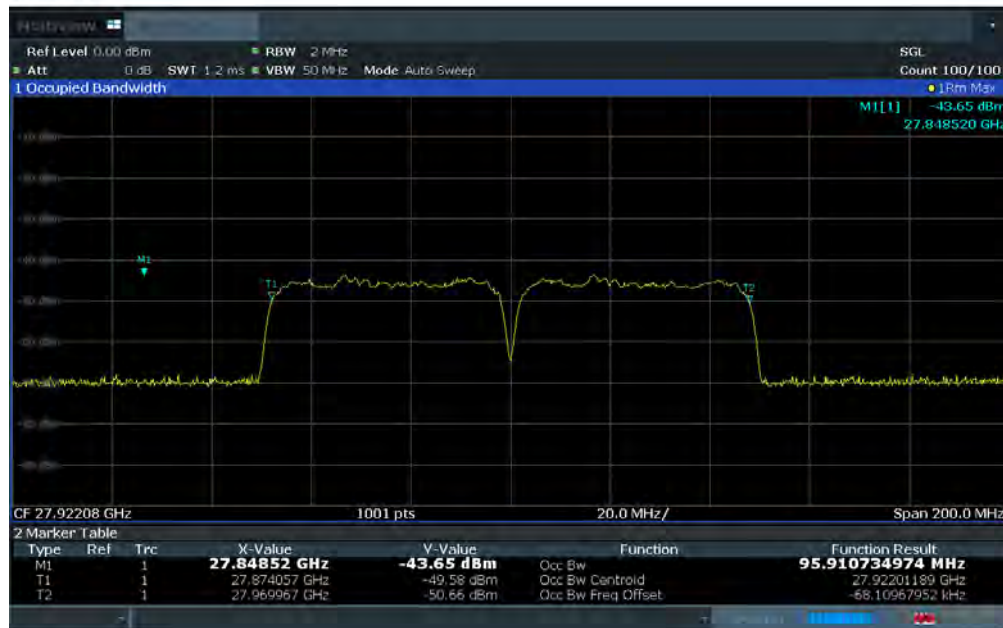
Plot 7-7. Ant 1 Occupied Bandwidth Plot (50MHz-2CC – 64QAM – Mid Channel)
