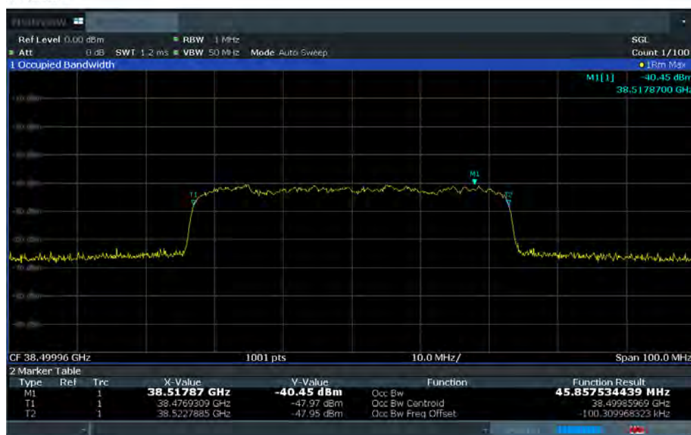
Plot 7-17. Ant 1 Occupied Bandwidth Plot (50MHz-1CC – QPSK – Mid Channel)
