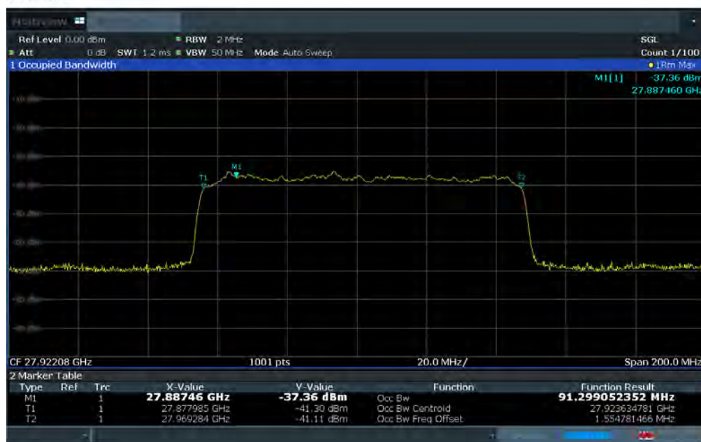
Plot 7-12. Ant 1 Occupied Bandwidth Plot (100MHz-1CC – pi/2-BPSK – Mid Channel)
