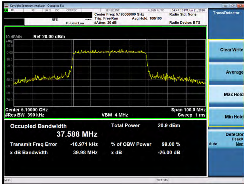
Plot 7-67. 26dB Bandwidth Plot SISO ANT2 (40MHz BW 802.11ax – 484 Tones (UNII Band 1) – Ch. 38)
