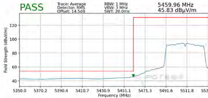
Plot 7-324. Radiated Lower Band Edge Plot MIMO (Average – UNII Band 2C)
