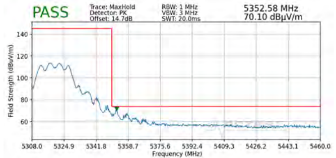
Plot 7-316. Radiated Upper Band Edge Plot MIMO (Peak – UNII Band 2A)
