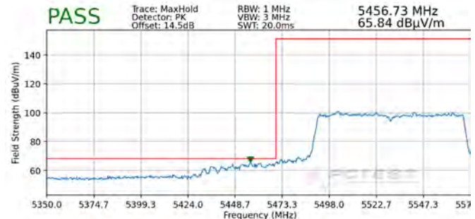
Plot 7-332. Radiated Lower Band Edge Plot MIMO (Peak – UNII Band 2C)
