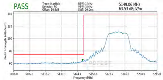
Plot 7-321. Radiated Lower Band Edge Plot MIMO (Peak – UNII Band 1)
