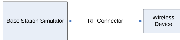
Figure 9-1 Power Measurement Setup
