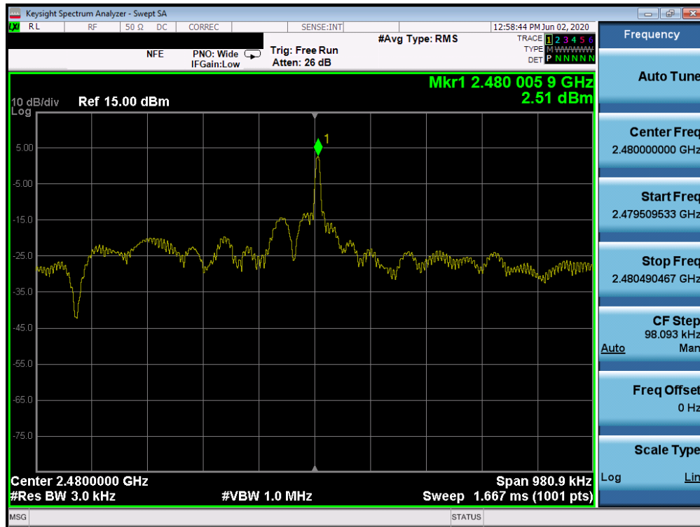
Plot 7-36. Power Spectral Density Plot (Bluetooth (LE), 2Mbps – Ch. 39)
