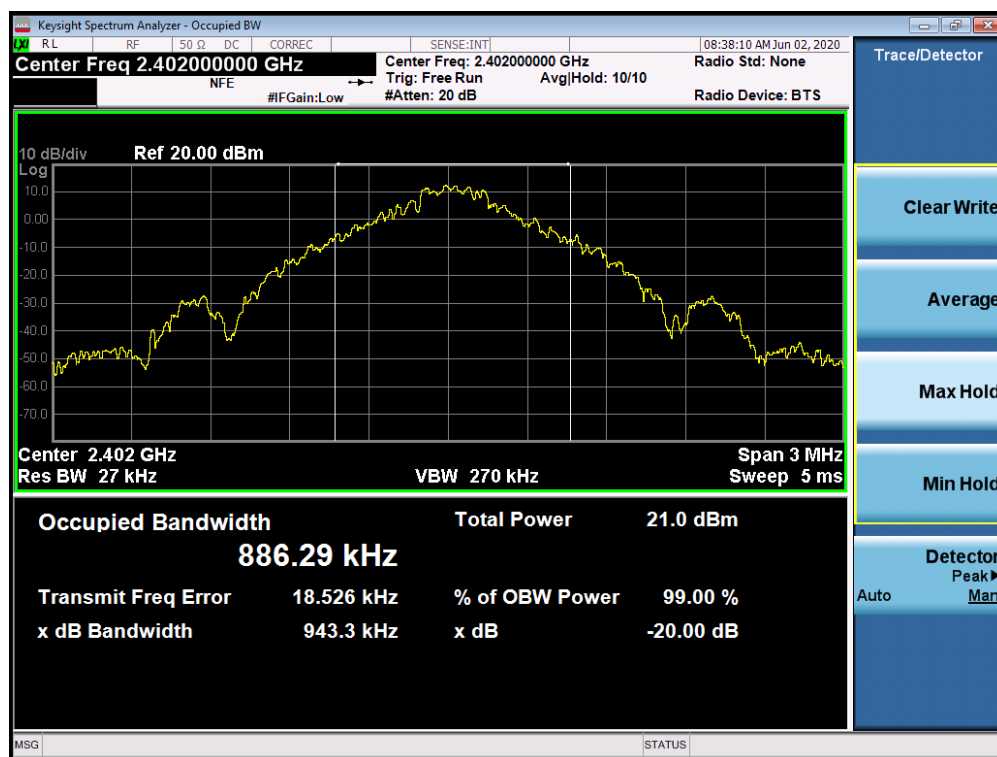
Plot 7-1. 20dB Bandwidth Plot (Bluetooth, 1Mbps – Ch. 0)
