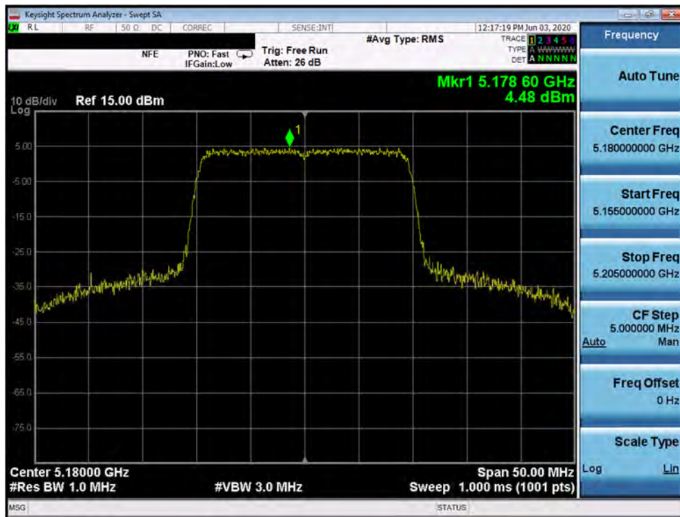
Plot 7-199. Power Spectral Density Plot SISO ANT2 (20MHz BW 802.11ax (UNII Band 1) – Ch. 36)
