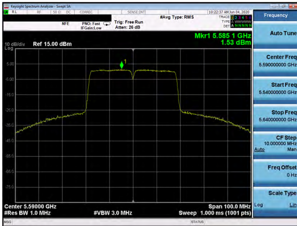
Plot 7-233. Power Spectral Density Plot SISO ANT2 (40MHz BW 802.11n (UNII Band 2C) – Ch. 118)
