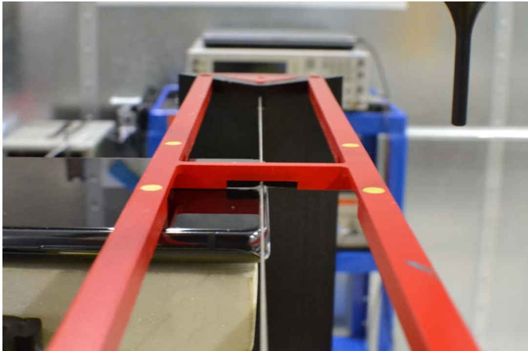
Figure 18-2 HAC Phantom Plane Alignment
