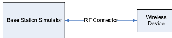
Figure 9-2 Power Measurement Setup
