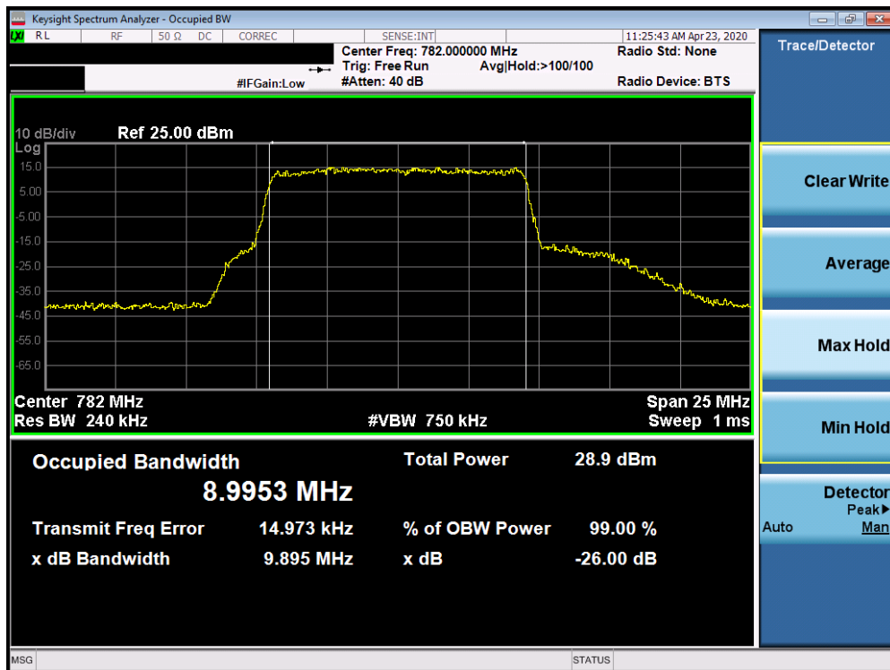
Plot 7-75. Occupied Bandwidth Plot (Band 13 - 10.0MHz 256-QAM - Full RB Configuration)
