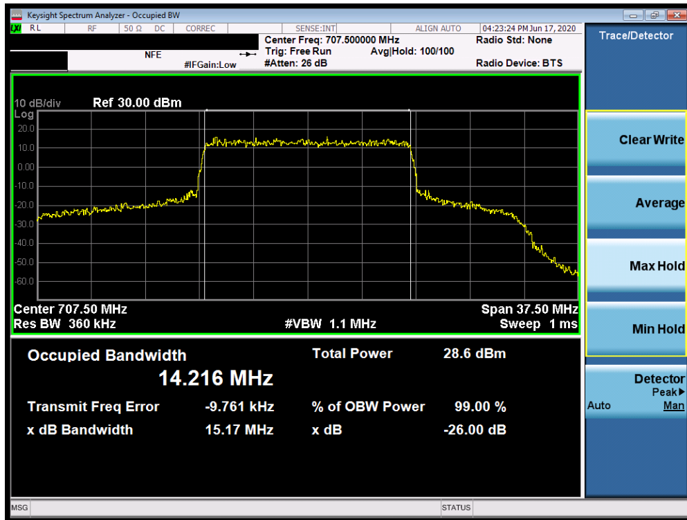
Plot 7-65. Occupied Bandwidth Plot (n12 15MHz 16QAM-CP-OFDM - Full RB Configuration)
