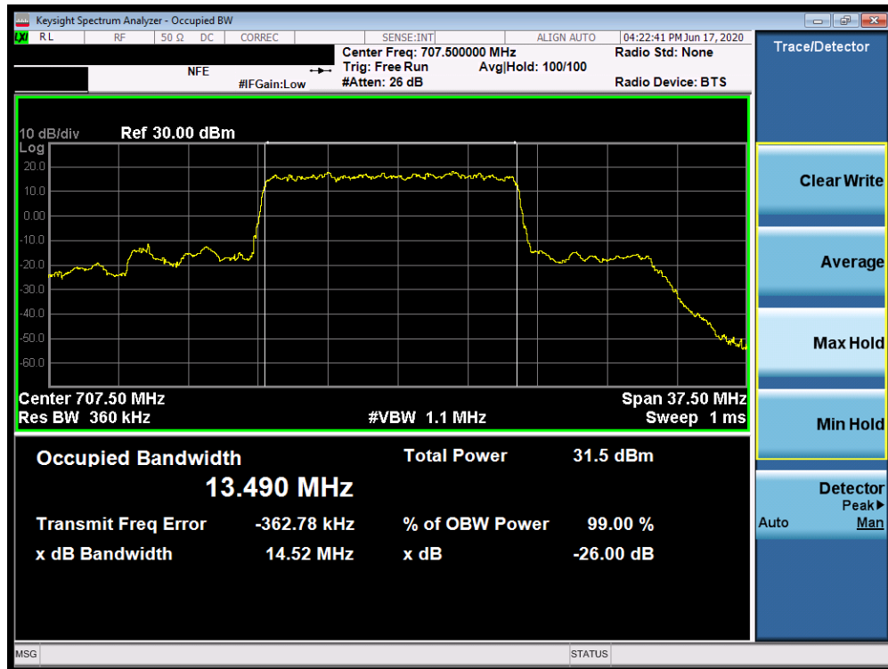
Plot 7-63. Occupied Bandwidth Plot (n12 15MHz BPSK-DFT-s-OFDM - Full RB Configuration)
