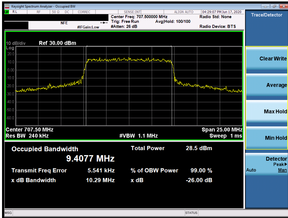
Plot 7-61. Occupied Bandwidth Plot (n12 10MHz 64QAM-CP-OFDM- Full RB Configuration)
