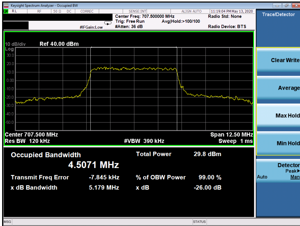
Plot 7-55. Occupied Bandwidth Plot (n12 5MHz 16QAM-CP-OFDM - Full RB Configuration)
