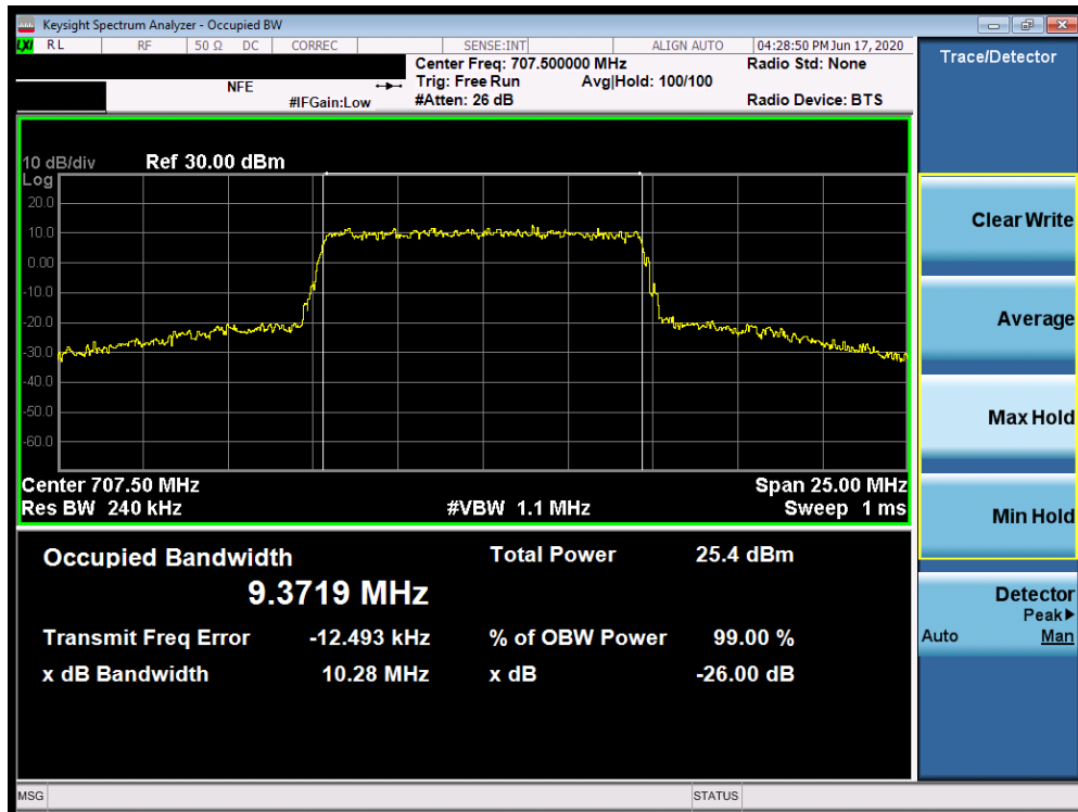
Plot 7-62. Occupied Bandwidth Plot (n12 10MHz 256QAM-CP-OFDM- Full RB Configuration)
