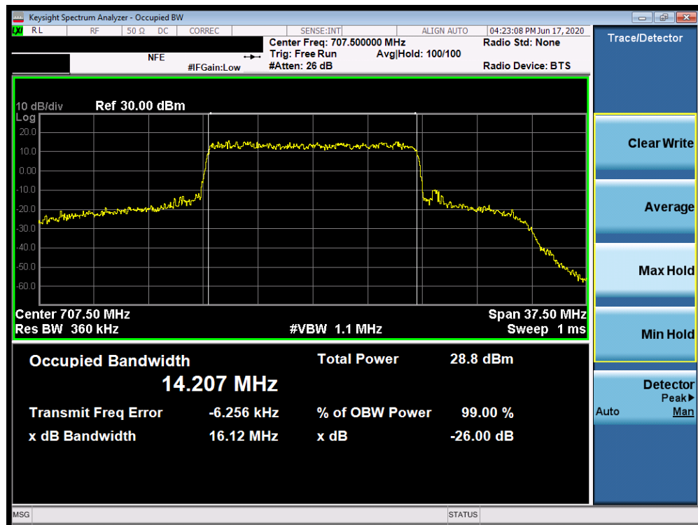
Plot 7-64. Occupied Bandwidth Plot (n12 15MHz QPSK-CP-OFDM - Full RB Configuration)
