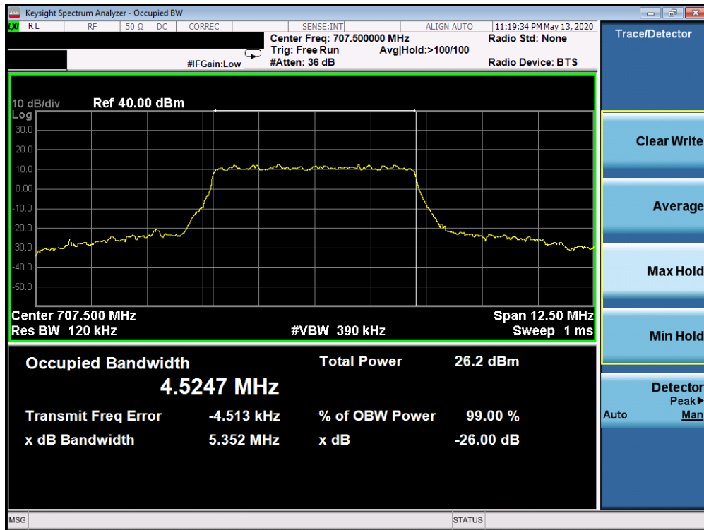
Plot 7-57. Occupied Bandwidth Plot (n12 5MHz 256QAM-CP-OFDM- Full RB Configuration)
