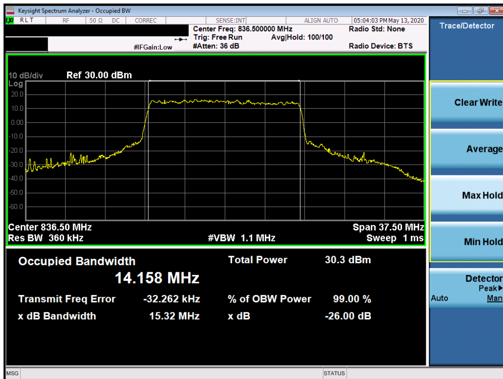
Plot 7-107. Occupied Bandwidth Plot (n5 15MHz QPSK-CP-OFDM - Full RB Configuration)
