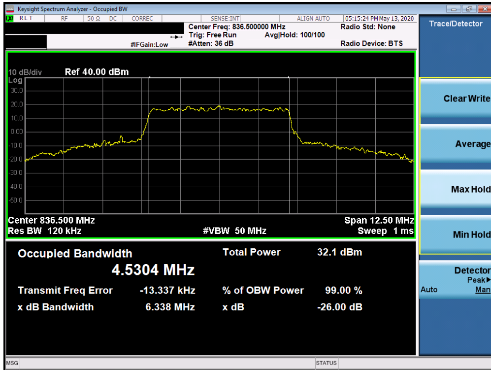
Plot 7-98. Occupied Bandwidth Plot (n5 5MHz 16QAM-CP-OFDM - Full RB Configuration)
