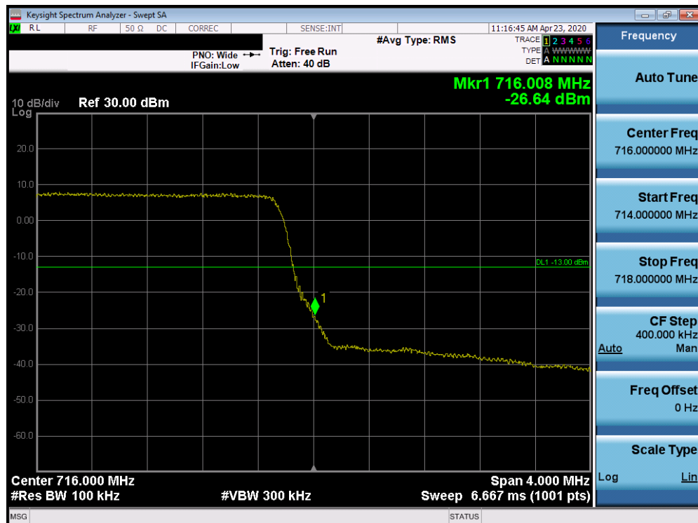
Plot 7-423. Upper Band Edge Plot (Band 12 - 5.0MHz QPSK - Full RB Configuration)
