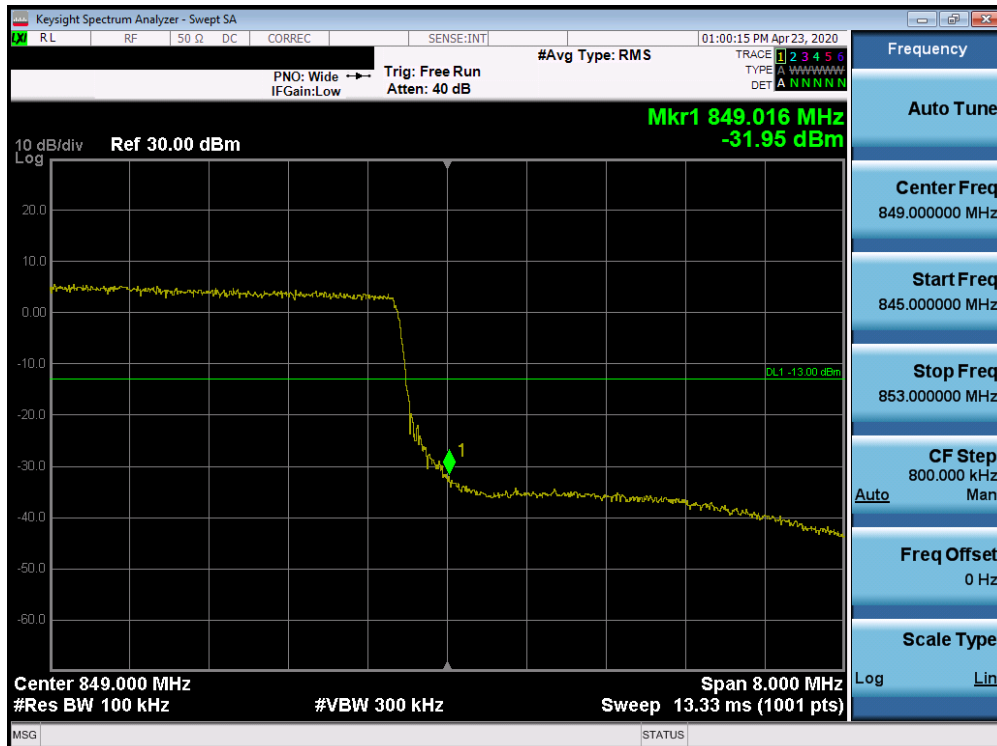
Plot 7-447. Upper Band Edge Plot (Band 26/5 - 10.0MHz QPSK - Full RB Configuration)
