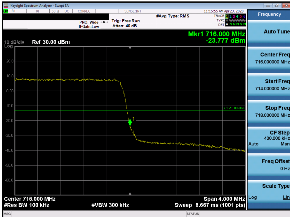
Plot 7-421. Upper Band Edge Plot (Band 12 - 3.0MHz QPSK - Full RB Configuration)
