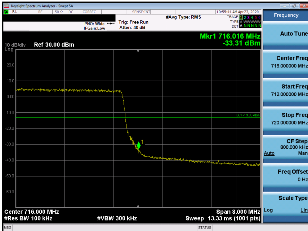
Plot 7-425. Upper Band Edge Plot (Band 12 - 10.0MHz QPSK - Full RB Configuration)
