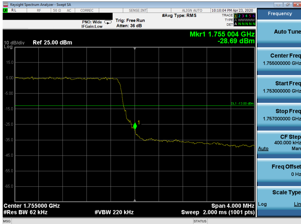
Plot 7-472. Upper Band Edge Plot (Band 4 - 5.0MHz QPSK - Full RB Configuration)
