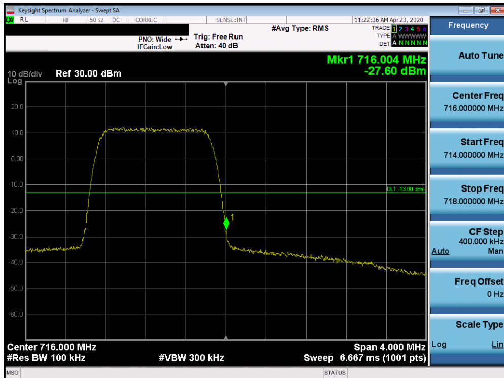
Plot 7-419. Upper Band Edge Plot (Band 12 - 1.4MHz QPSK - Full RB Configuration)
