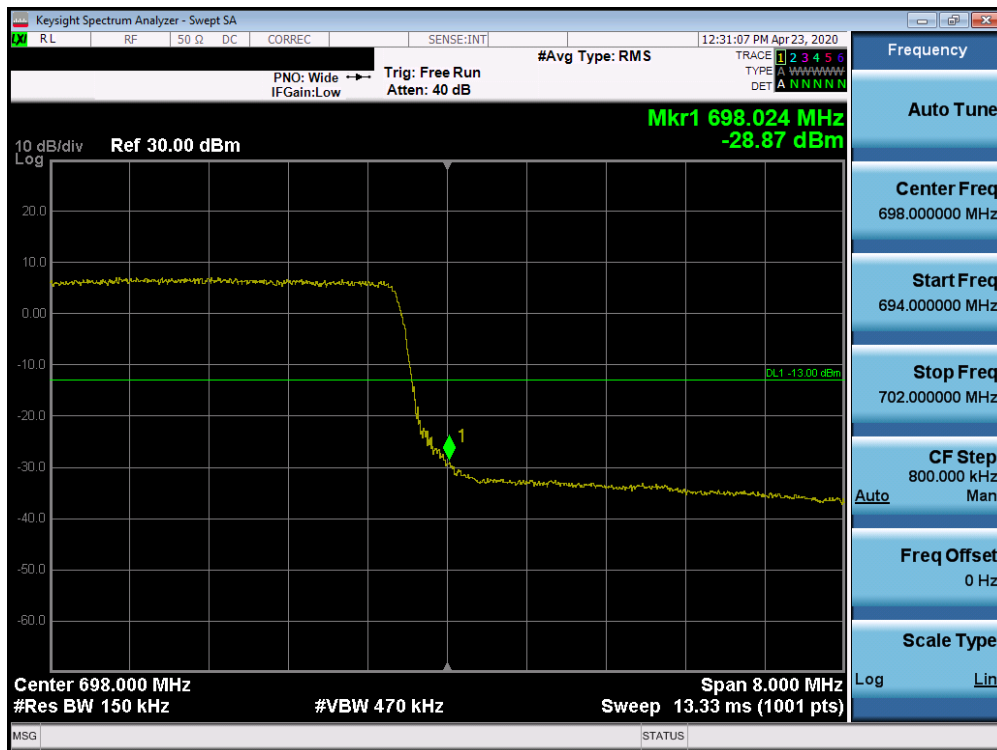
Plot 7-405. Upper Band Edge Plot (Band 71 - 10.0MHz QPSK - Full RB Configuration)
