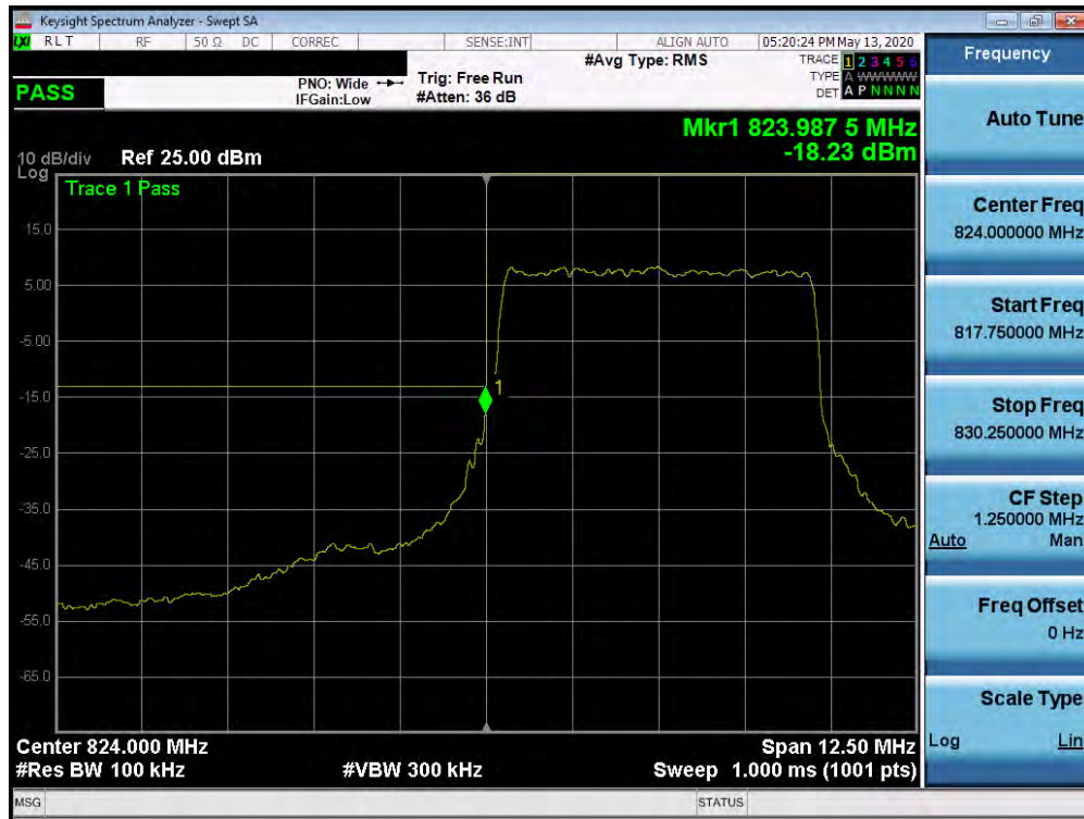
Plot 7-450. Lower Band Edge Plot (n5 – 5.0MHz DFT-s-OFDM BPSK - Full RB Configuration)
