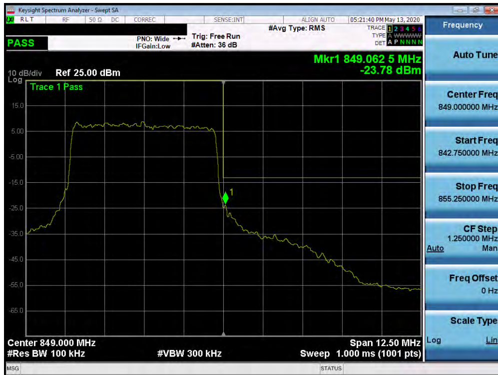
Plot 7-451. Upper Band Edge Plot (n5 – 5.0MHz DFT-s-OFDM BPSK - Full RB Configuration)
