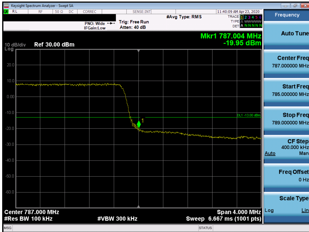
Plot 7-434. Upper Band Edge Plot (Band 13 - 5.0MHz QPSK - Full RB Configuration)
