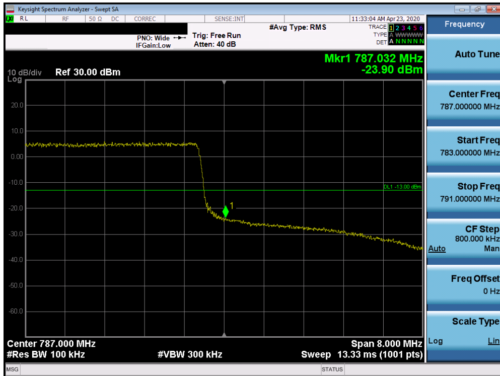
Plot 7-438. Upper Band Edge Plot (Band 13 - 10.0MHz QPSK - Full RB Configuration)
