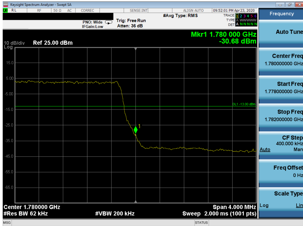
Plot 7-474. Upper Band Edge Plot (Band 66 - 5.0MHz QPSK - Full RB Configuration)
