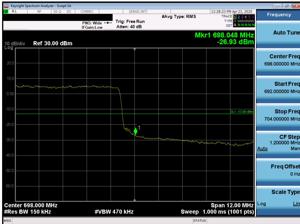
Plot 7-407. Upper Band Edge Plot (Band 71 - 15.0MHz QPSK - Full RB Configuration)
