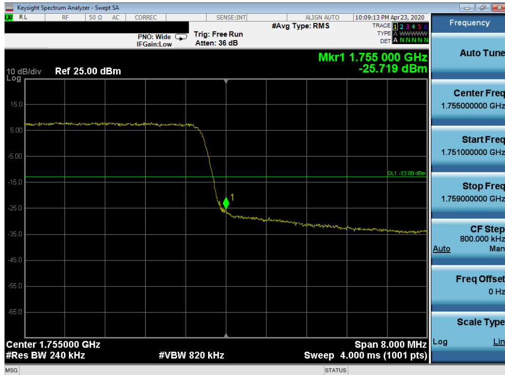
Plot 7-478. Upper Band Edge Plot (Band 4 - 10.0MHz QPSK - Full RB Configuration)
