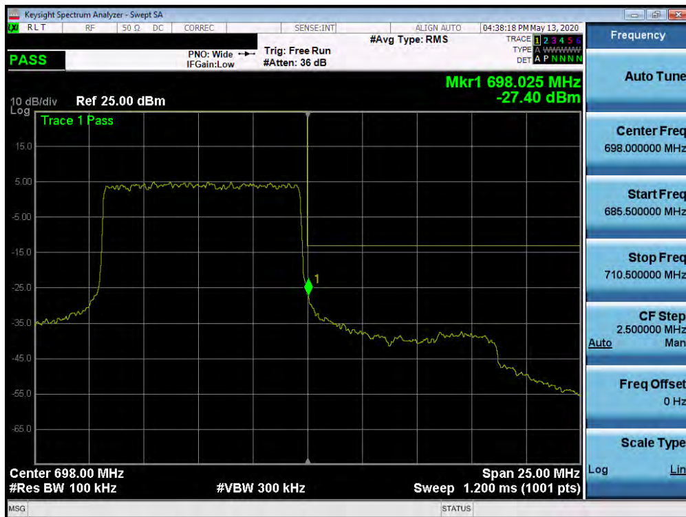
Plot 7-413. Upper Band Edge Plot (n71 - 10MHz DFT-s-OFDM-QPSK - Full RB Configuration)
