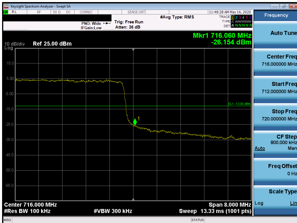
Plot 7-429. Upper Band Edge Plot (n12 - 10MHz DFT-s-OFDM-QPSK - Full RB Configuration)
