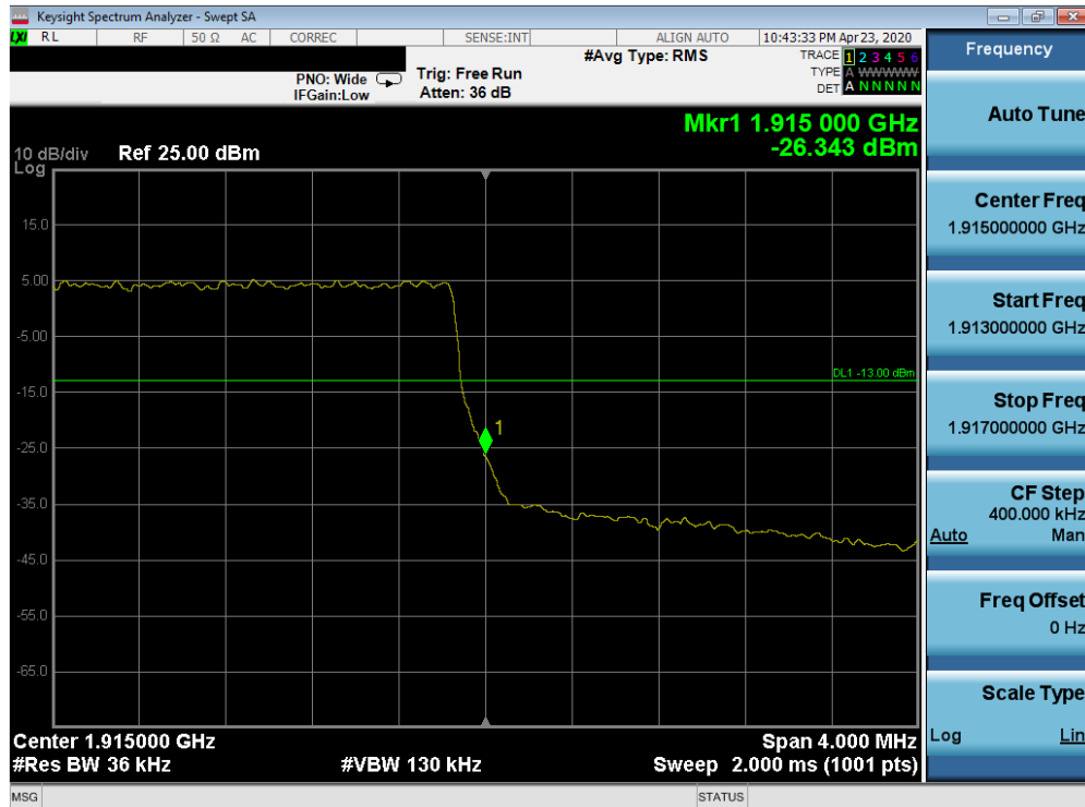
Plot 7-520. Upper Band Edge Plot (Band 25 - 3.0MHz QPSK - Full RB Configuration)
