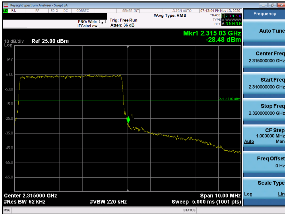
Plot 7-572. Upper Band Edge Plot (Band 30 - 5.0MHz QPSK - Full RB Configuration)
