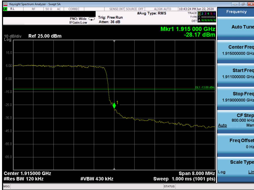
Plot 7-556. Upper Band Edge Plot (n25 - 10MHz DFT-s-OFDM-QPSK - Full RB Configuration)
