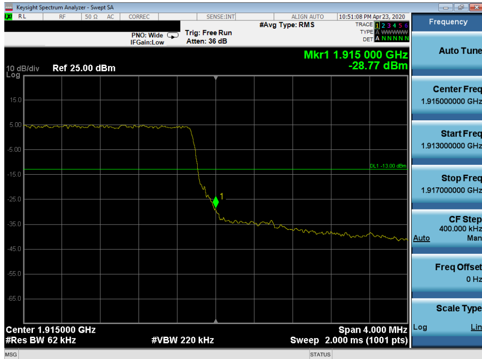
Plot 7-526. Upper Band Edge Plot (Band 25 - 5.0MHz QPSK - Full RB Configuration)
