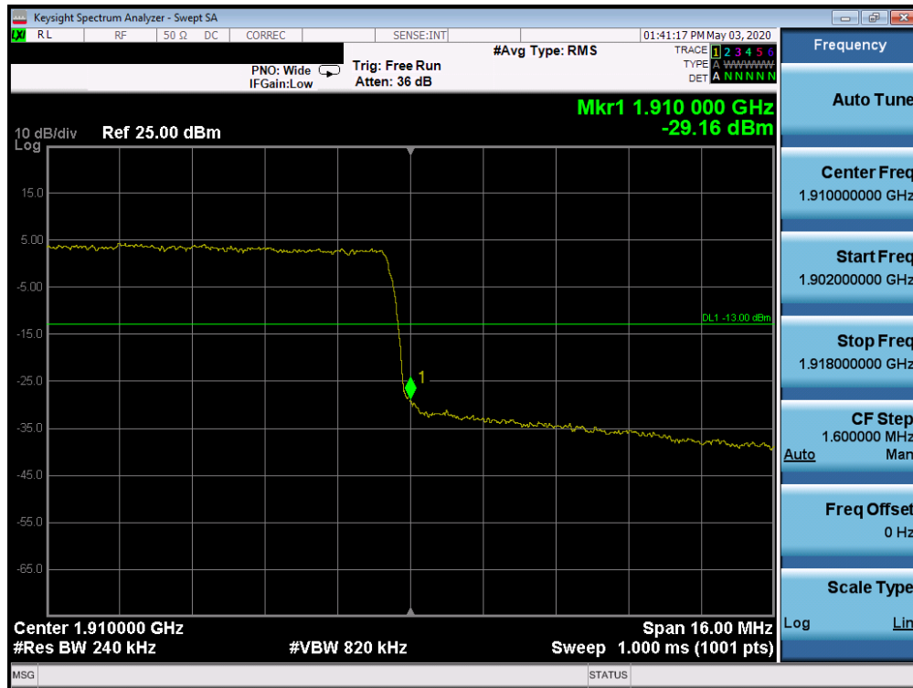
Plot 7-566. Upper Band Edge Plot (n2 - 20MHz DFT-s-OFDM-QPSK - Full RB Configuration)
