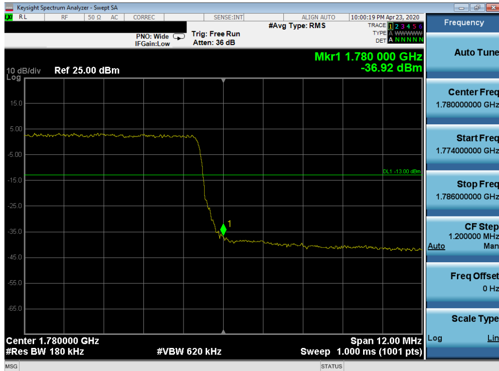
Plot 7-486. Upper Band Edge Plot (Band 66 - 15.0MHz QPSK - Full RB Configuration)
