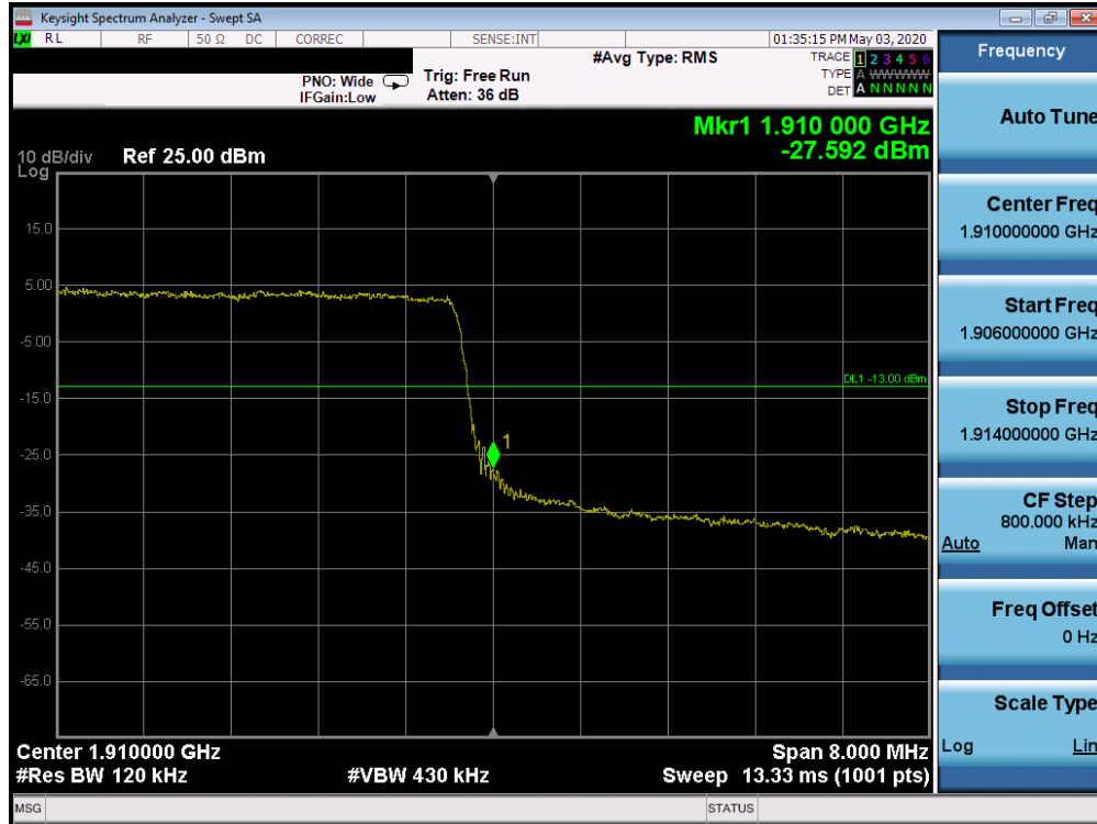
Plot 7-554. Upper Band Edge Plot (n2 - 10MHz DFT-s-OFDM-QPSK - Full RB Configuration)
