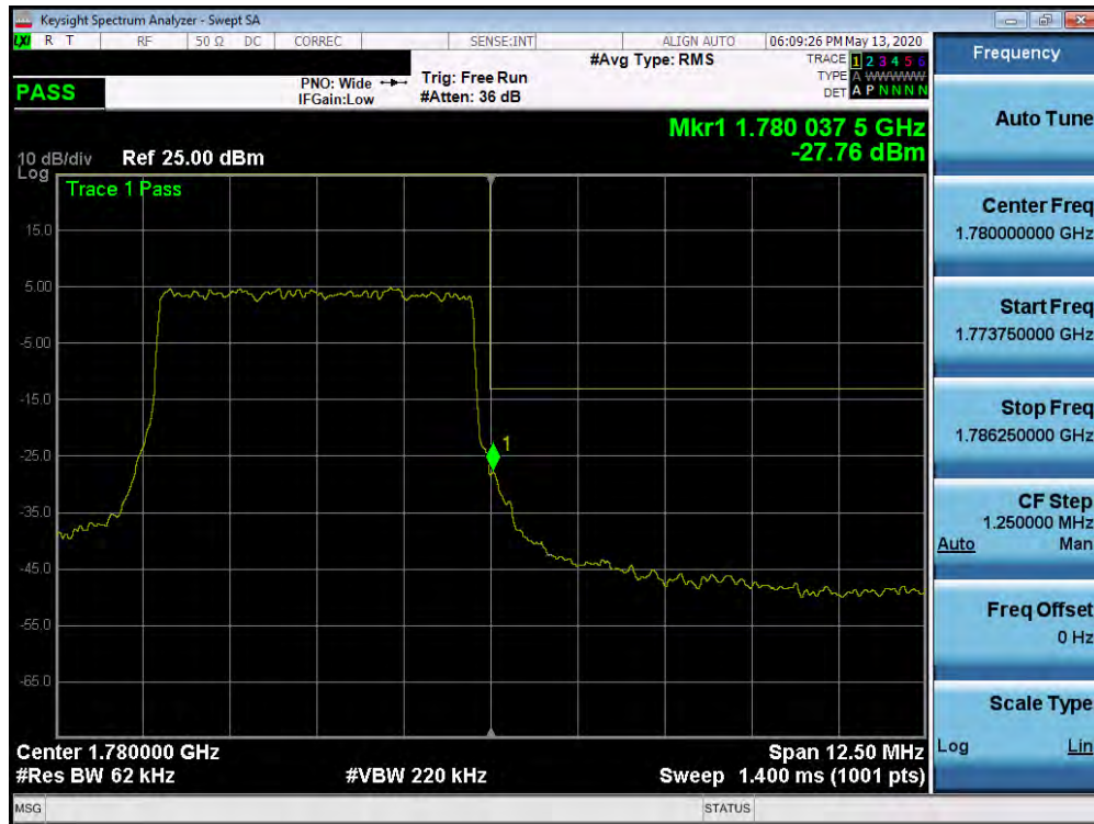
Plot 7-496. Upper Band Edge Plot (n66 - 5MHz DFT-s-OFDM-QPSK - Full RB Configuration)
