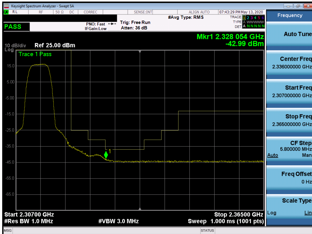
Plot 7-573. Upper Extended Band Edge Plot (Band 30 - 5.0MHz QPSK - Full RB Configuration)
