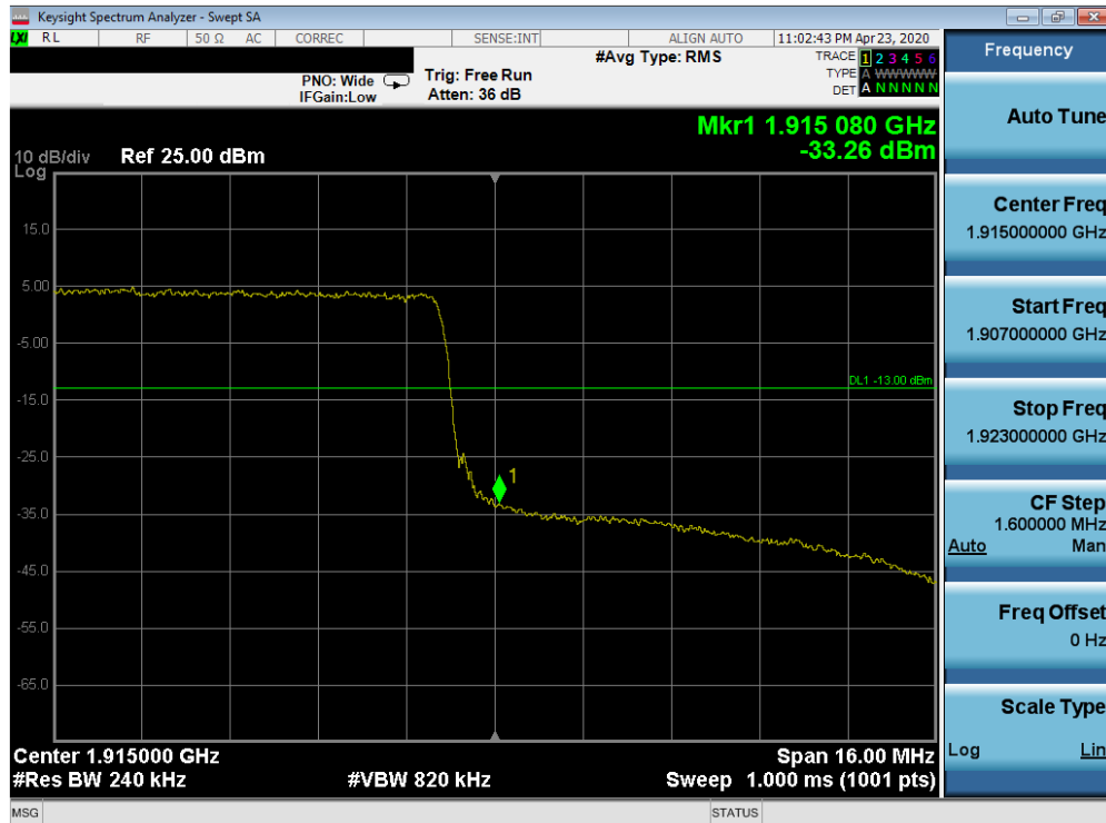
Plot 7-544. Upper Band Edge Plot (Band 25 - 20.0MHz QPSK - Full RB Configuration)
