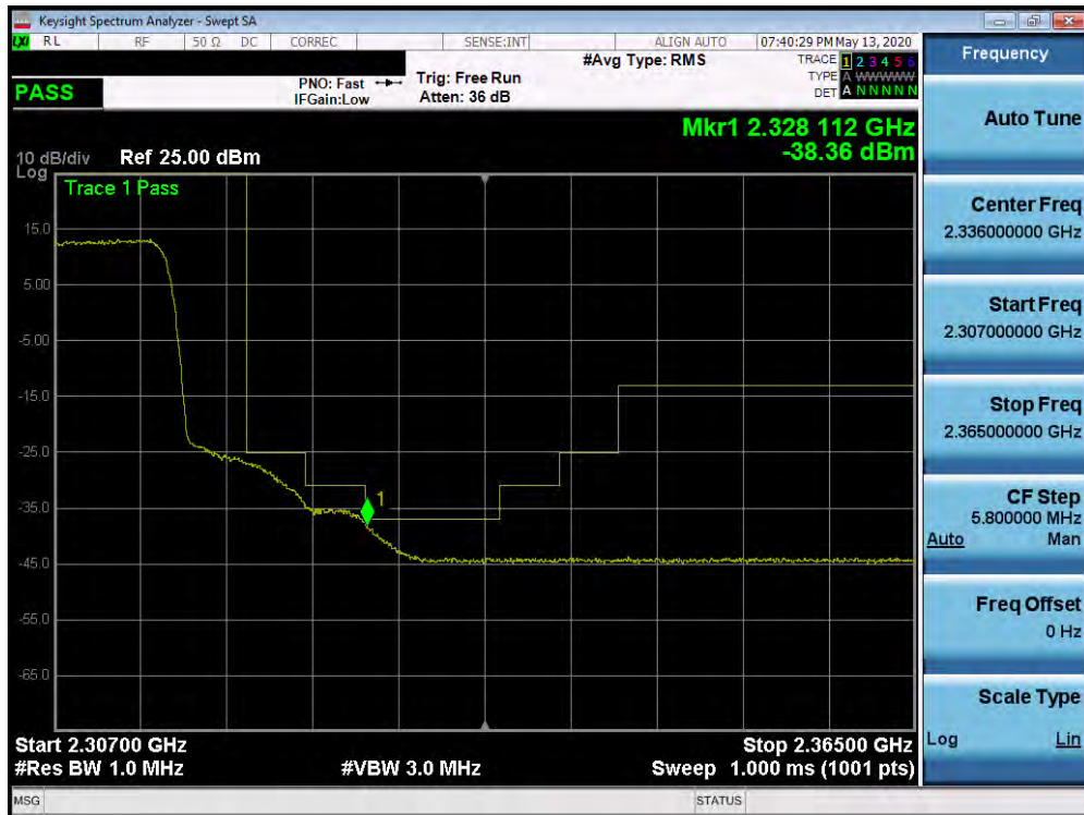
Plot 7-577. Upper Extended Band Edge Plot (Band 30 - 10.0MHz QPSK - Full RB Configuration)
