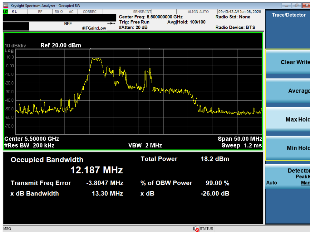
Plot 7-55. 26dB Bandwidth Plot SISO ANT2 (20MHz BW 802.11ax – 26 Tones (UNII Band 2C) – Ch. 100)
