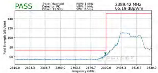
Plot 7-82. Radiated Restricted Lower Band Edge Measurement SISO ANT1 (Peak – 106 Tones)
