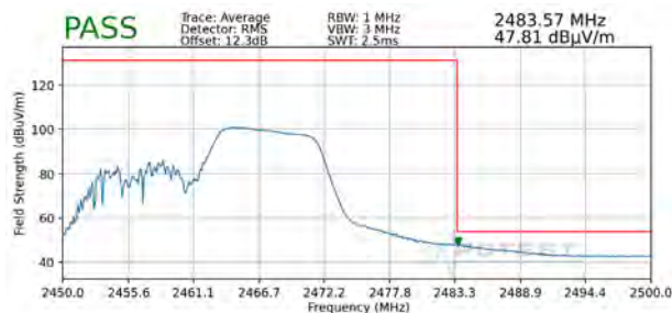
Plot 7-107. Radiated Restricted Upper Band Edge Measurement MIMO (Average – 106 Tones)
