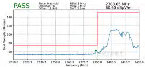
Plot 7-106. Radiated Restricted Lower Band Edge Measurement MIMO (Peak – 106 Tones)
