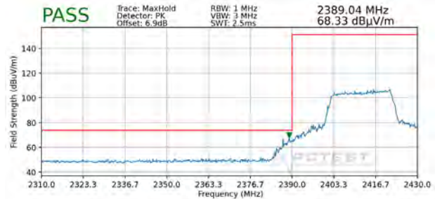
Plot 7-86. Radiated Restricted Lower Band Edge Measurement SISO ANT1 (Peak - 242 Tones)
