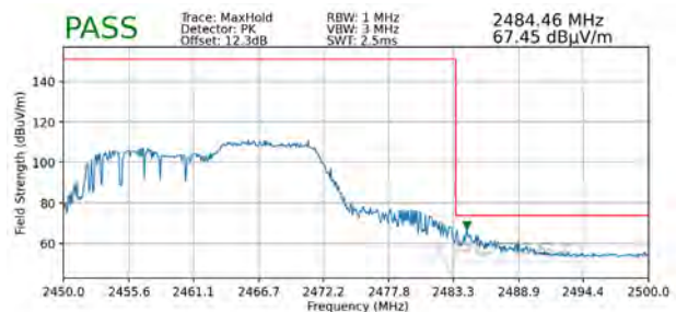
Plot 7-84. Radiated Restricted Upper Band Edge Measurement SISO ANT1 (Peak – 106 Tones)
