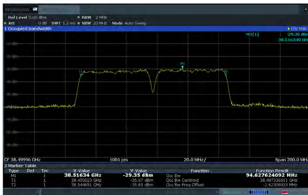
Plot 7-22. Ant 2 Occupied Bandwidth Plot (50MHz-2CC – 16QAM – Mid Channel)
