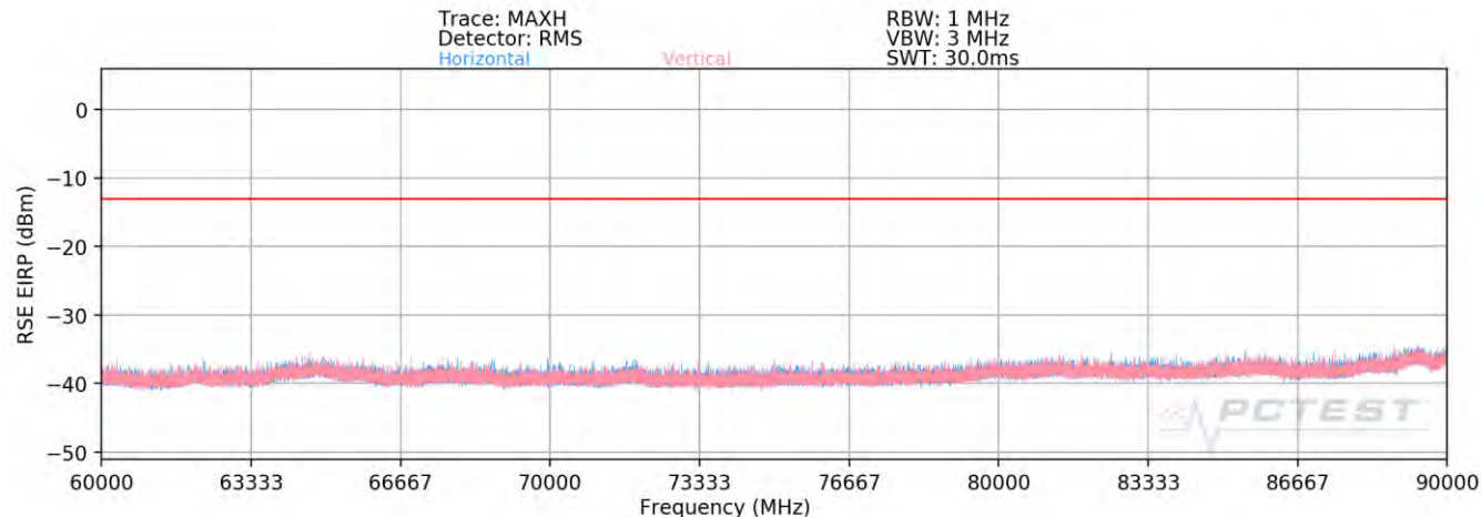
Plot 7-38. Ant 1-n261 Radiated Spurious Plot (1CC QPSK Mid Channel V Beam – ENDC Anchor B2)
