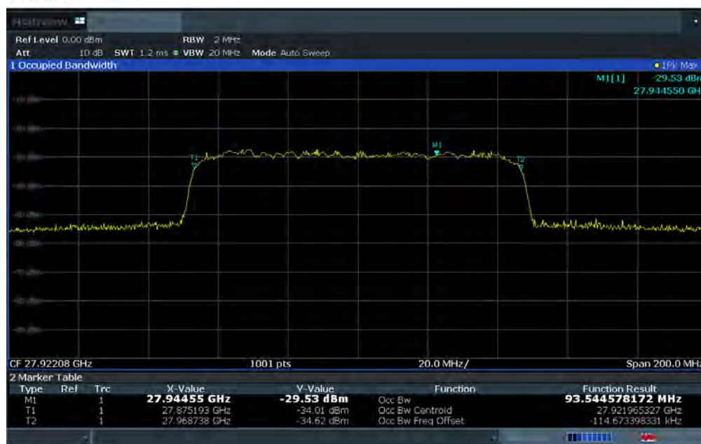
Plot 7-10. Ant 2 Occupied Bandwidth Plot (100MHz-1CC – 16QAM – Mid Channel)
