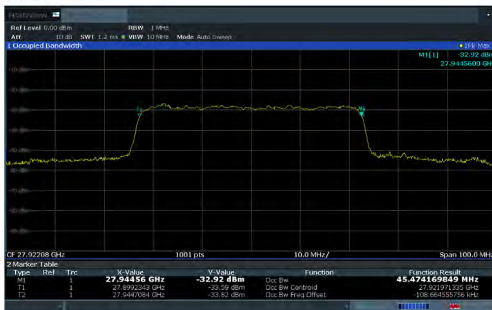
Plot 7-1. Ant 2 Occupied Bandwidth Plot (50MHz-1CC – QPSK – Mid Channel)
