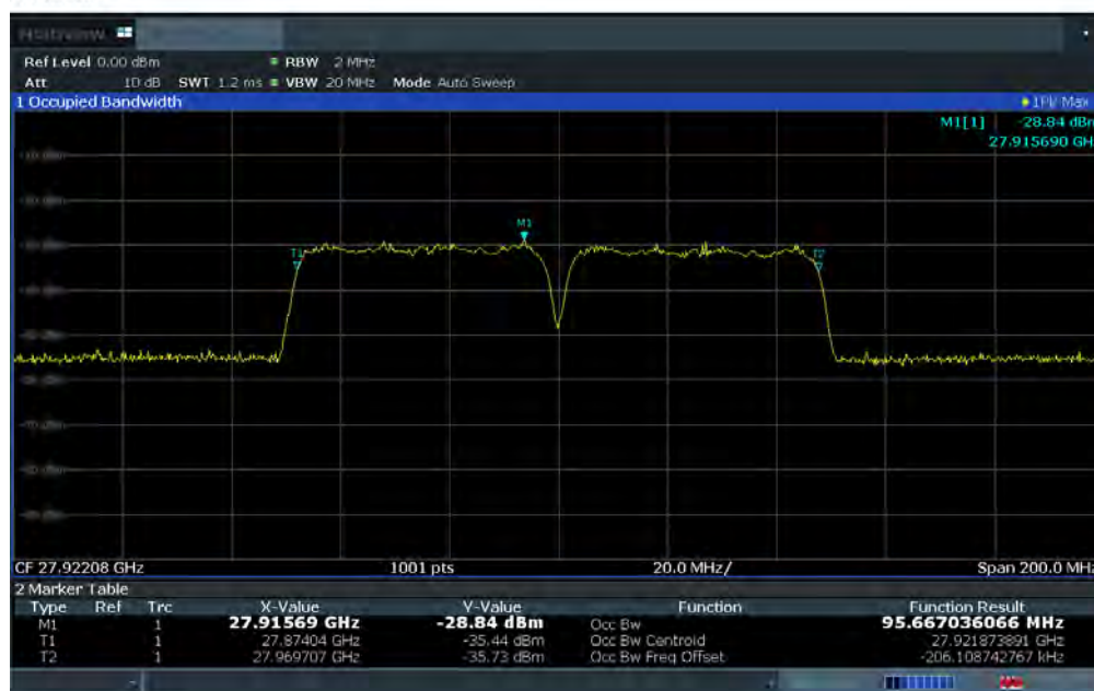
Plot 7-7. Ant 2 Occupied Bandwidth Plot (50MHz-2CC – 64QAM – Mid Channel)
