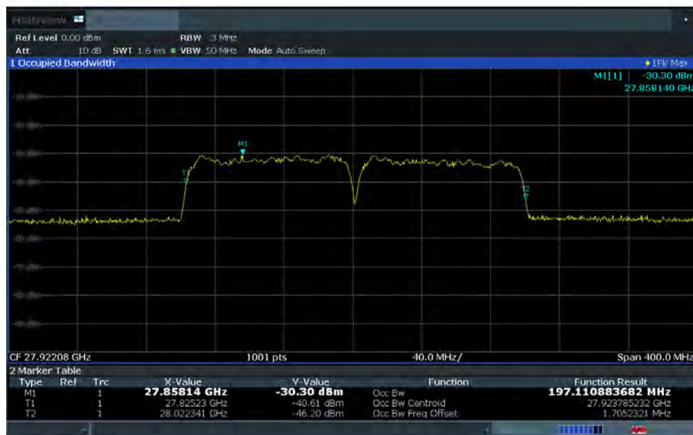
Plot 7-13. Ant 2 Occupied Bandwidth Plot (100MHz-2CC – QPSK – Mid Channel)
