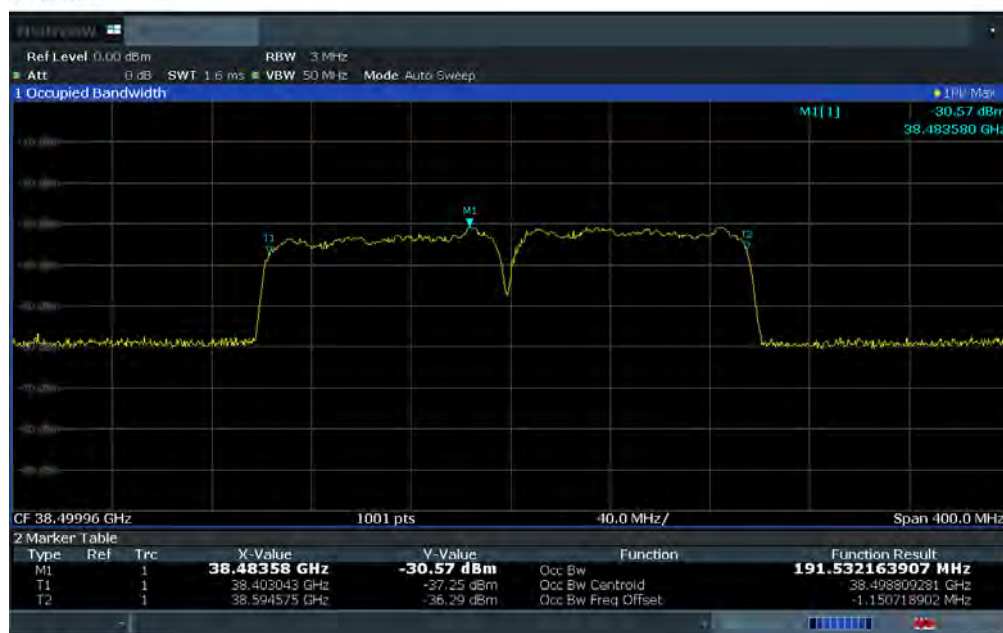
Plot 7-30. Ant 2 Occupied Bandwidth Plot (100MHz-2CC – 16QAM – Mid Channel)
