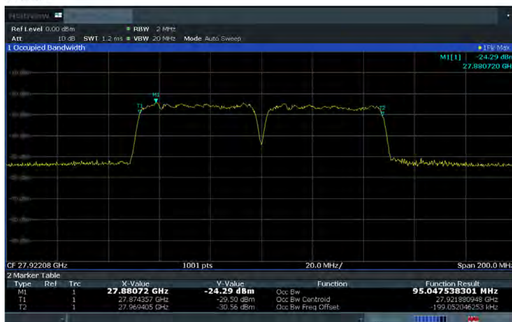
Plot 7-5. Ant 2 Occupied Bandwidth Plot (50MHz-2CC – QPSK – Mid Channel)
