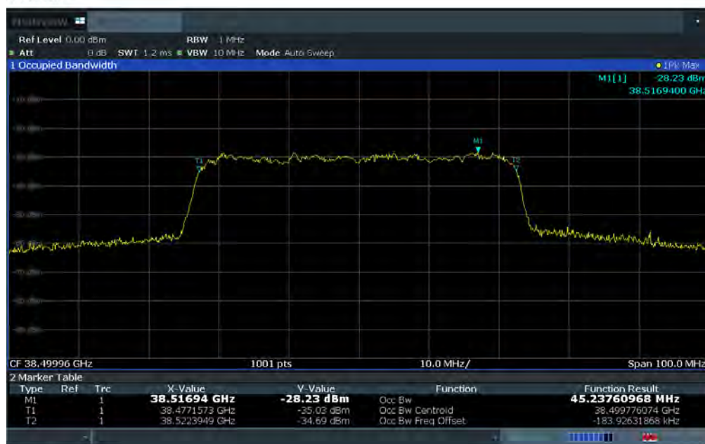
Plot 7-18. Ant 2 Occupied Bandwidth Plot (50MHz-1CC – 16QAM – Mid Channel)
