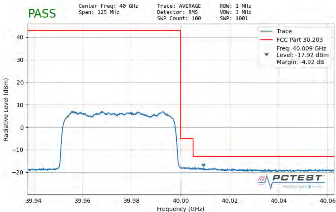
Plot 7-89. Ant 2 Upper Band Edge (50MHz-1CC – QPSK Full RB)
