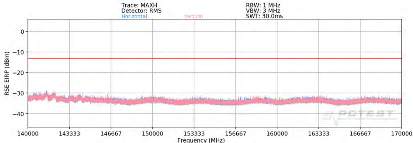
Plot 7-53. Ant 1-n260 Radiated Spurious Plot (1CC QPSK Mid Channel MIMO – ENDC Anchor Band 2)
