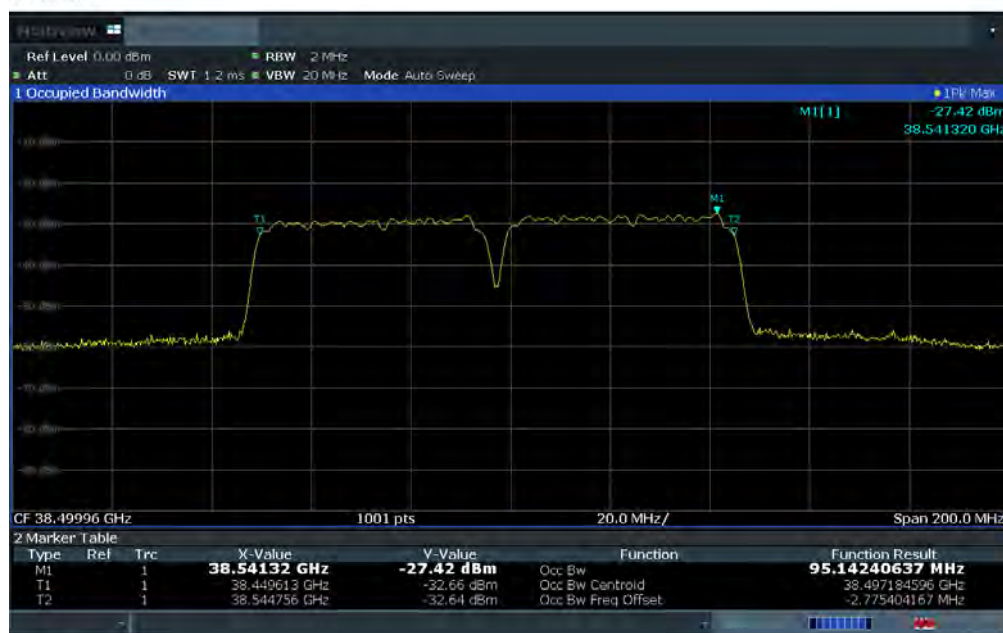
Plot 7-24. Ant 2 Occupied Bandwidth Plot (50MHz-2CC – pi/2-BPSK – Mid Channel)
