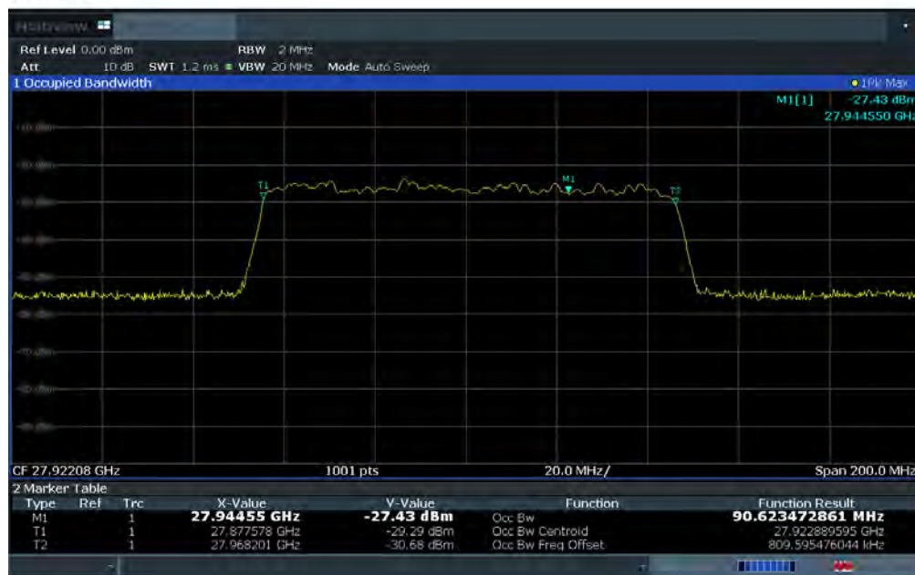
Plot 7-12. Ant 2 Occupied Bandwidth Plot (100MHz-1CC – pi/2-BPSK – Mid Channel)
