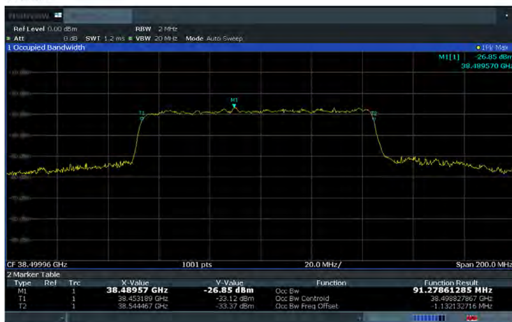
Plot 7-25. Ant 2 Occupied Bandwidth Plot (100MHz-1CC – QPSK – Mid Channel)
