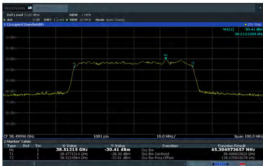
Plot 7-19. Ant 2 Occupied Bandwidth Plot (50MHz-1CC – 64QAM – Mid Channel)
