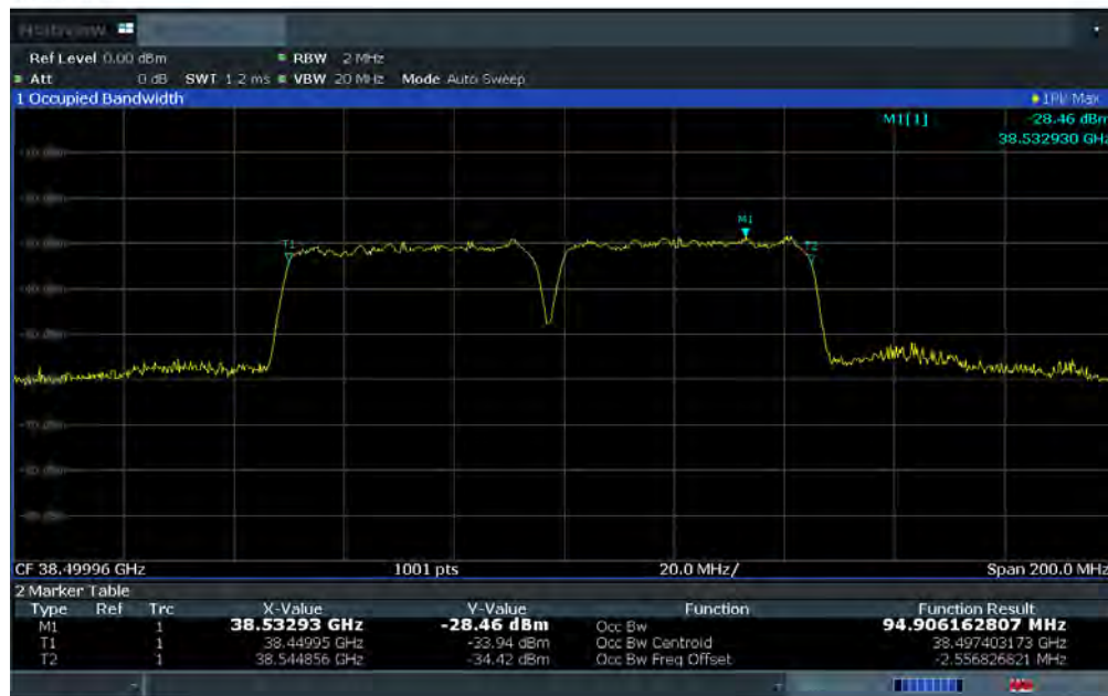
Plot 7-21. Ant 2 Occupied Bandwidth Plot (50MHz-2CC – QPSK – Mid Channel)
