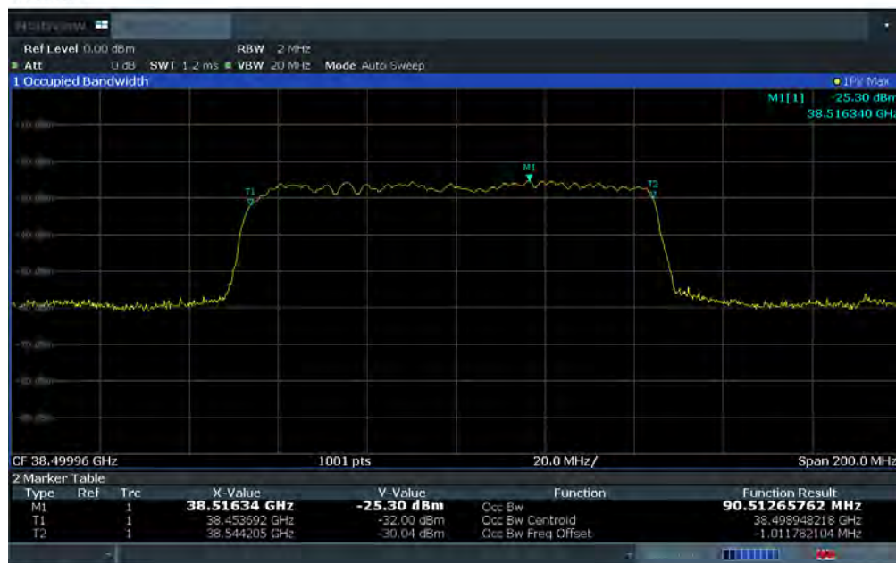
Plot 7-28. Ant 2 Occupied Bandwidth Plot (100MHz-1CC – pi/2-BPSK – Mid Channel)
