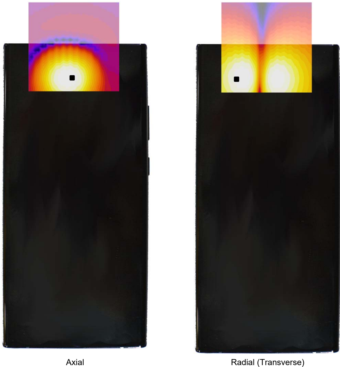
Figure 16-3 T-Coil Scan Overlay Magnetic Field Distributions
