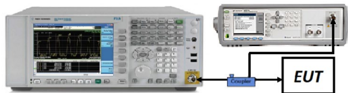
Figure 7-6. Test Instrument & Measurement Setup
