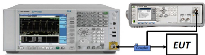
Figure 7-5. Test Instrument & Measurement Setup
