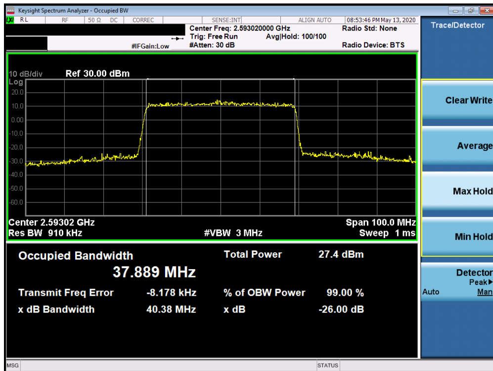
Plot 7-194. Occupied Bandwidth Plot (n41 40MHz 256QAM-CP-OFDM- Full RB Configuration)
