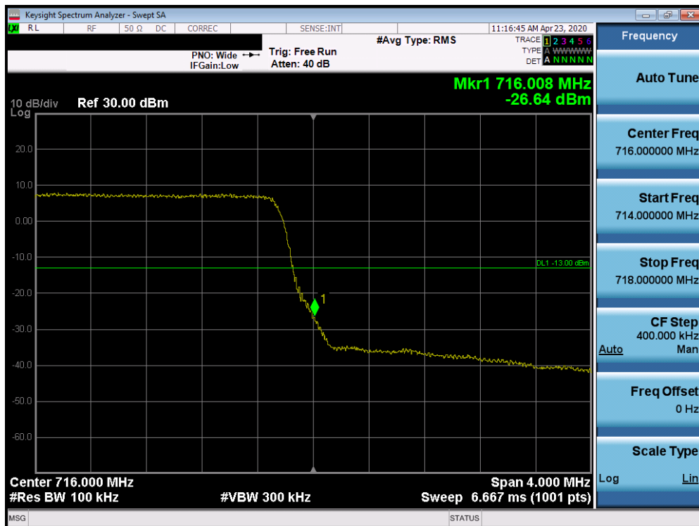
Plot 7-328. Upper Band Edge Plot (Band 12 - 5.0MHz QPSK - Full RB Configuration)
