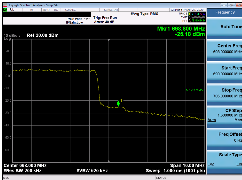
Plot 7-314. Upper Band Edge Plot (Band 71 - 20.0MHz QPSK - Full RB Configuration)
