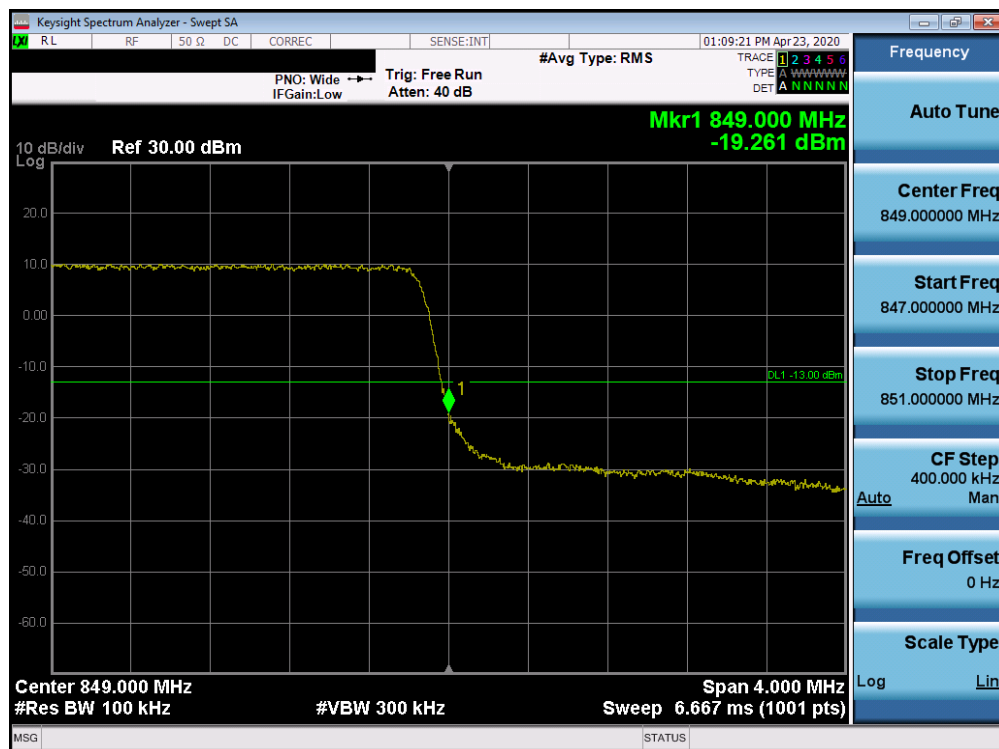
Plot 7-342. Upper Band Edge Plot (Band 5 - 3.0MHz QPSK - Full RB Configuration)
