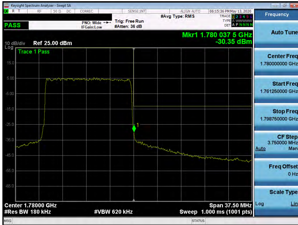
Plot 7-393. Upper Band Edge Plot (n66 - 15MHz DFT-s-OFDM-QPSK - Full RB Configuration)
