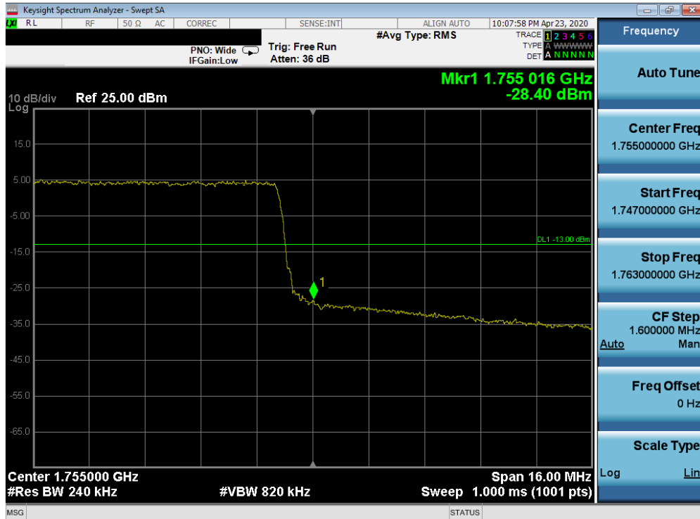
Plot 7-379. Upper Band Edge Plot (Band 4 - 20.0MHz QPSK - Full RB Configuration)
