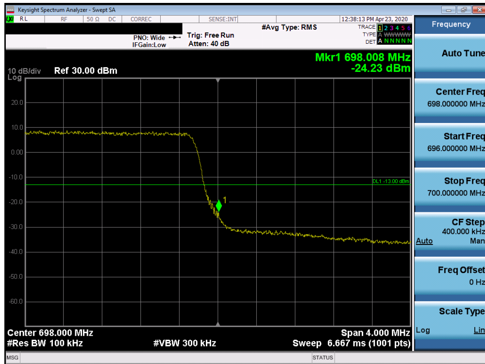
Plot 7-308. Upper Band Edge Plot (Band 71 - 5.0MHz QPSK - Full RB Configuration)
