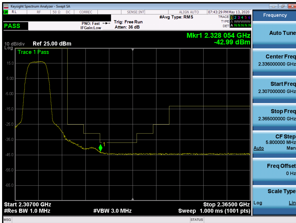
Plot 7-438. Upper Extended Band Edge Plot (Band 30 - 5.0MHz QPSK - Full RB Configuration)
