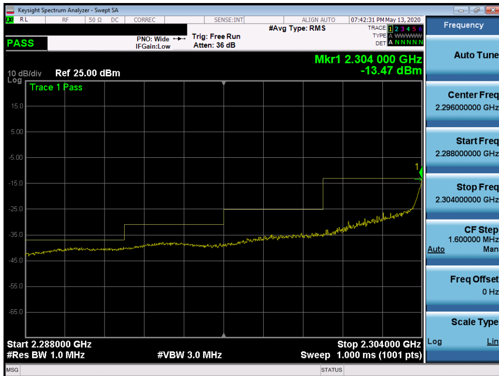
Plot 7-436. Lower Extended Band Edge Plot (Band 30 - 5.0MHz QPSK - Full RB Configuration)
