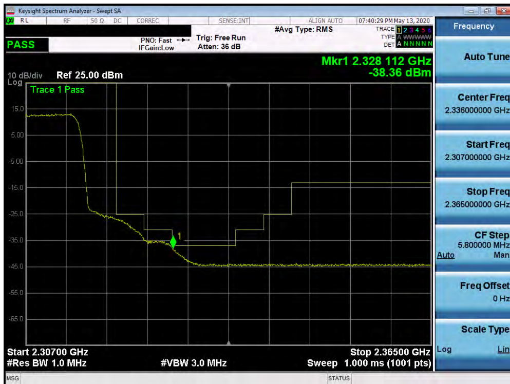
Plot 7-442. Upper Extended Band Edge Plot (Band 30 - 10.0MHz QPSK - Full RB Configuration)
