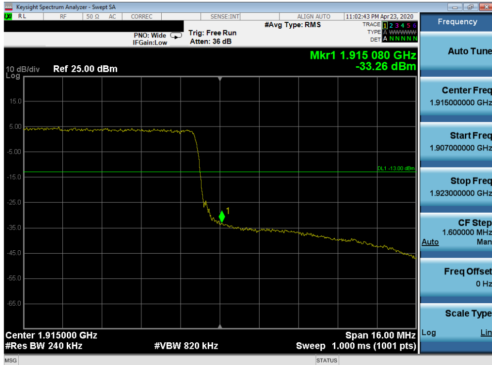
Plot 7-433. Upper Band Edge Plot (Band 25 - 20.0MHz QPSK - Full RB Configuration)
