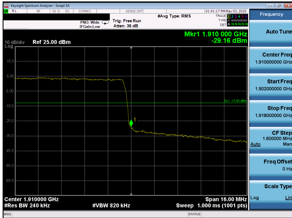
Plot 7-431. Upper Band Edge Plot (Band 2 - 20.0MHz QPSK - Full RB Configuration)
