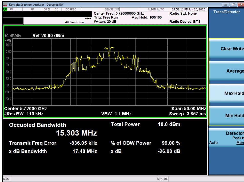
Plot 7-15. 26dB Bandwidth Plot SISO ANT1 (20MHz BW 802.11ax – 26 Tones (UNII Band 2C) – Ch. 144)
