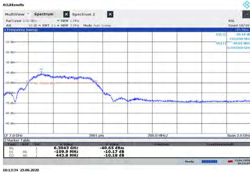
Plot 7-6. BANDWIDTH Plot - ANT1 - CH.5 – SP3 – Preamble 9
