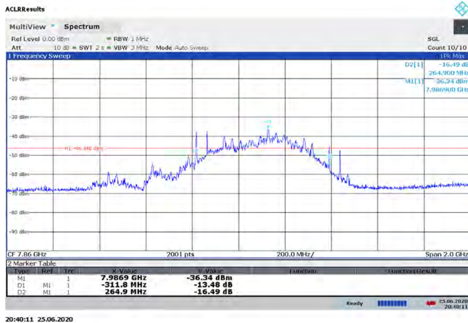
Plot 7-38. BANDWIDTH Plot - ANT1 - CH.9 – SP1 – Preamble 10
