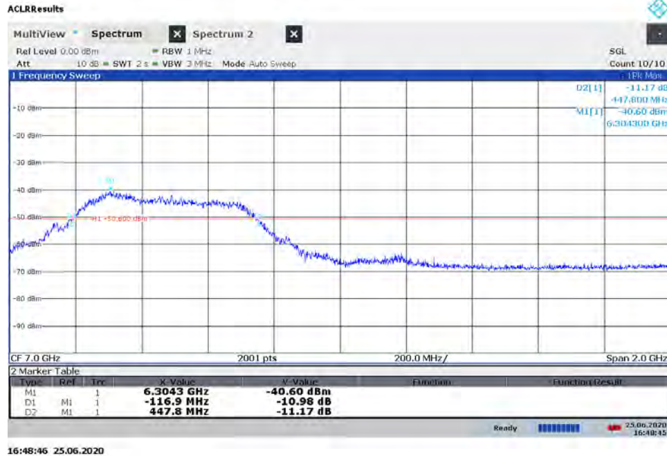
Plot 7-17. BANDWIDTH Plot – ANT2 - CH.5 – SP1 – Preamble 11
