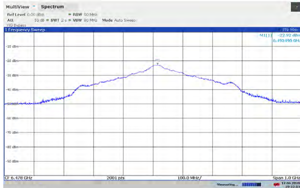
Plot 7-64. UWB Peak Power Measurement - ANT 1 - CH.5 – SP1 – BPRF
