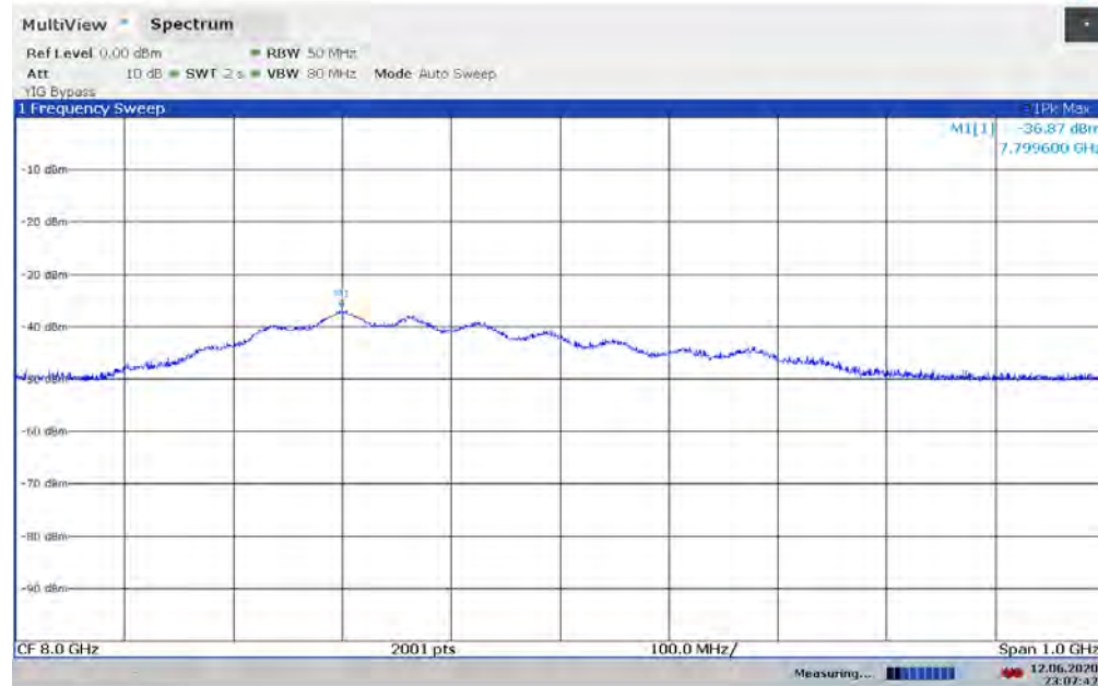
Plot 7-108. UWB Peak Power Measurement - ANT 2 - CH.9 – SP3 – HPRF
