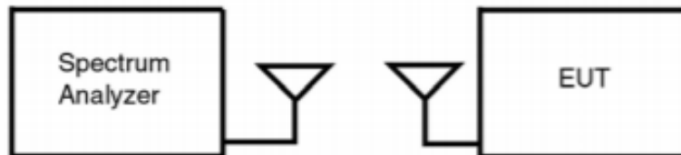
Figure 7-2. Test Instrument and Measurement Setup
