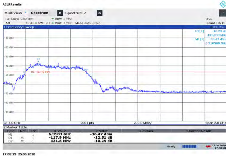
Plot 7-30. BANDWIDTH Plot – ANT2 - CH.5 – SP3 – Preamble 27
