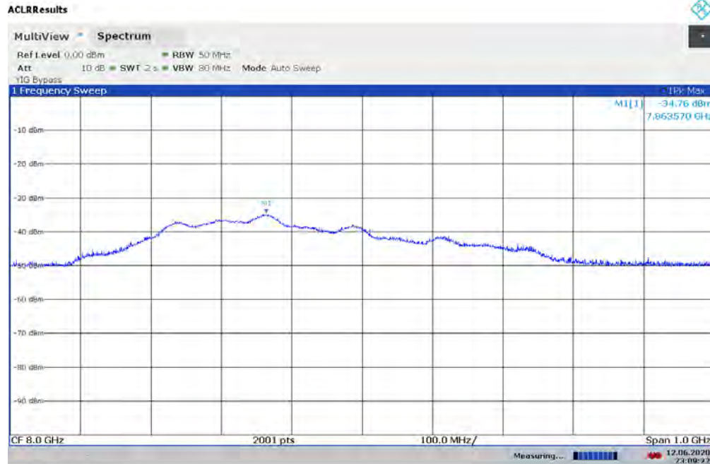
Plot 7-106. UWB Peak Power Measurement - ANT 2 - CH.9 – SP1 – HPRF
