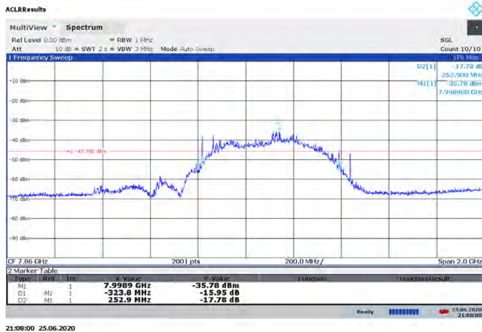
Plot 7-56. BANDWIDTH Plot – ANT1 - CH.9 – SP1 – Preamble 27
