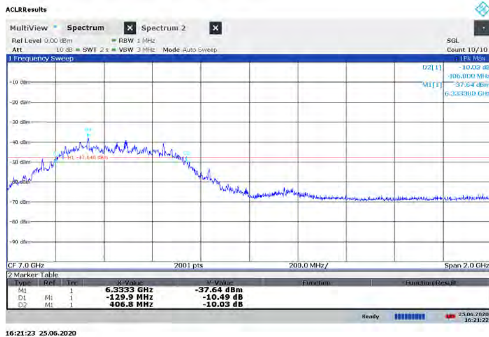
Plot 7-4. BANDWIDTH Plot – ANT2 - CH.5 - SP0 – Preamble 9
