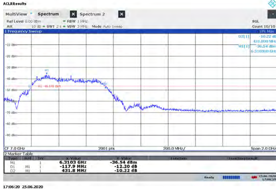
Plot 7-29. BANDWIDTH Plot – ANT2 - CH.5 – SP1 – Preamble 27
