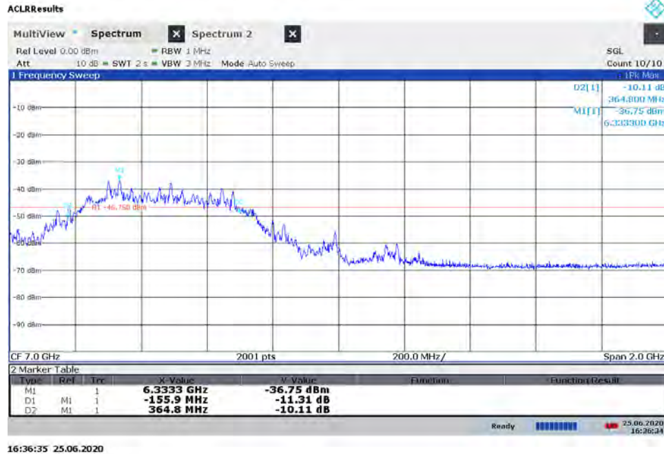
Plot 7-11. BANDWIDTH Plot – ANT2 - CH.5 – SP1 – Preamble 10
