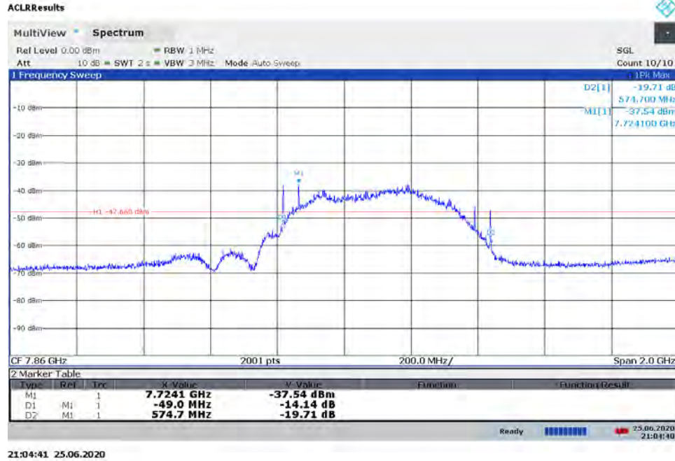
Plot 7-57. BANDWIDTH Plot – ANT1 - CH.9 – SP3 – Preamble 27
