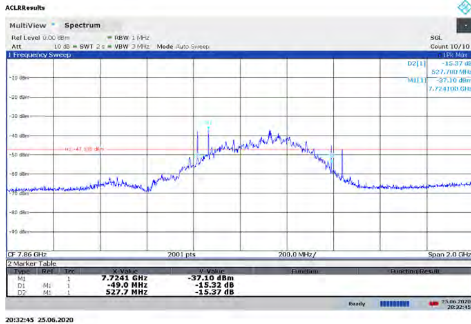
Plot 7-31. BANDWIDTH Plot - ANT1 - CH.9 - SP0 - Preamble 9
