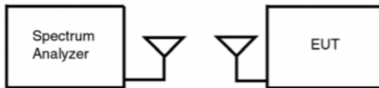
Figure 7-1. Test Instrument and Measurement Setup
