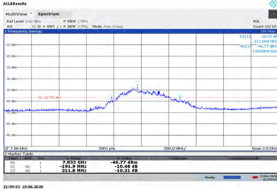
Plot 7-53. BANDWIDTH Plot – ANT2 - CH.9 – SP1 – Preamble 12
