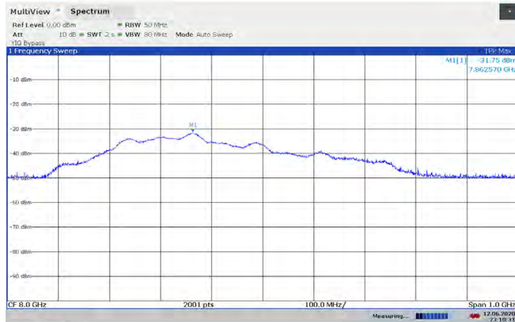
Plot 7-104. UWB Peak Power Measurement - ANT 2 - CH.9 - SP0 - HPRF
