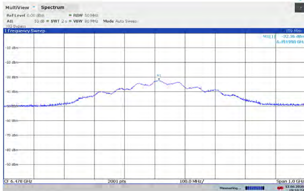
Plot 7-66. UWB Peak Power Measurement - ANT 1 - CH.5 – SP3 – BPRF
