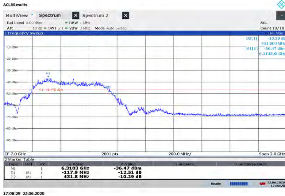
Plot 7-28. BANDWIDTH Plot – ANT2 - CH.5 - SP0 – Preamble 27
