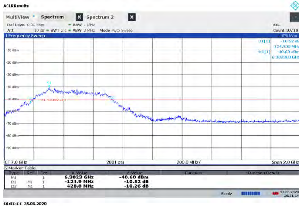
Plot 7-16. BANDWIDTH Plot – ANT2 - CH.5 - SP0 – Preamble 11
