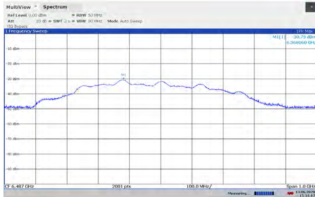
Plot 7-100. UWB Peak Power Measurement - ANT 2 - CH.5 – SP1 – HPRF
