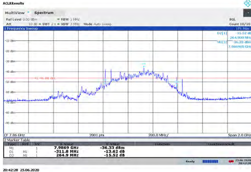
Plot 7-37. BANDWIDTH Plot - ANT1 - CH.9 - SP0 – Preamble 10
