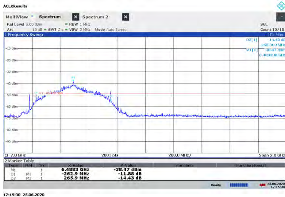
Plot 7-26. BANDWIDTH Plot – ANT1 - CH.5 – SP1 – Preamble 27
