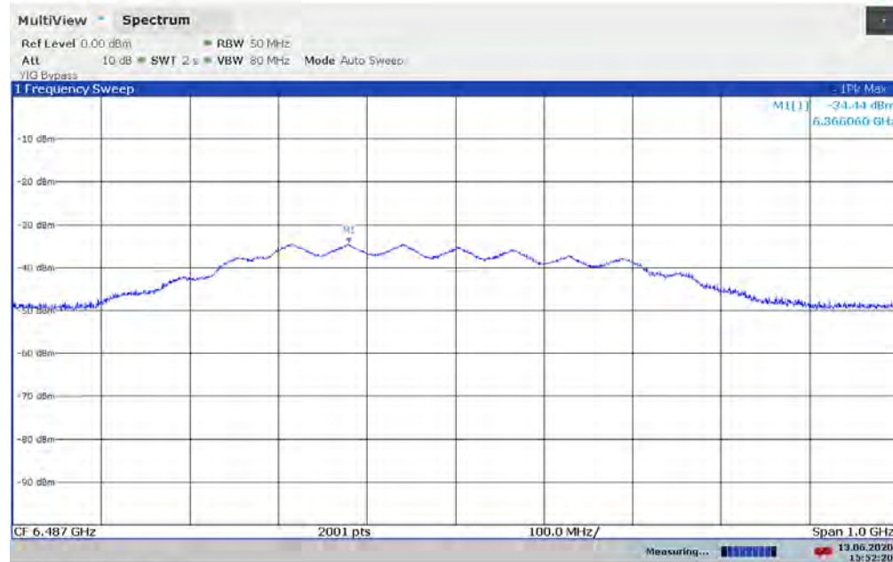
Plot 7-102. UWB Peak Power Measurement - ANT 2 - CH.5 – SP3 – HPRF
