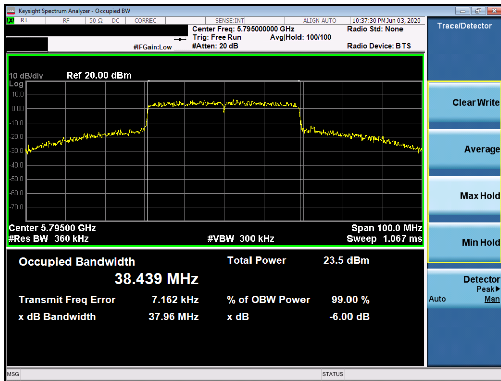
Plot 7-124. 6dB Bandwidth Plot SISO ANT2 (40MHz BW 802.11ax (UNII Band 3) – Ch. 159)
