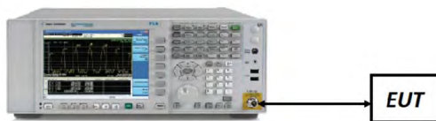
Figure 7-4. Test Instrument & Measurement Setup
