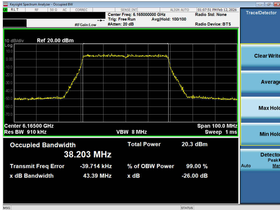
Plot 7-3. 26dB Bandwidth Plot SISO ANT1 (40MHz 802.11ax (UNII Band 5) – Ch. 43) - LPI
