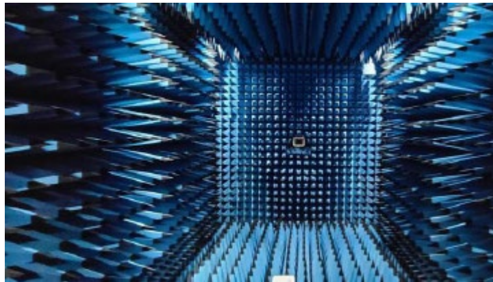
Figure 1: Geometry of Anechoic Chamber for Radiation patterns.
