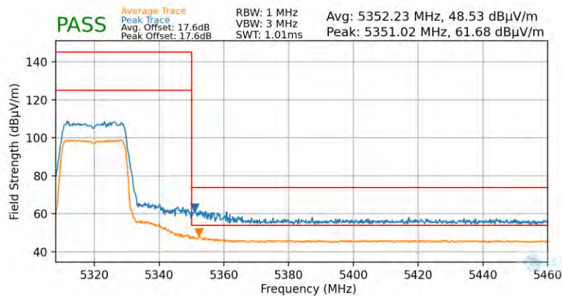
Plot 7-80. Radiated Upper Band Edge Plot (Average & Peak – UNII Band 2A – 242 Tones)
