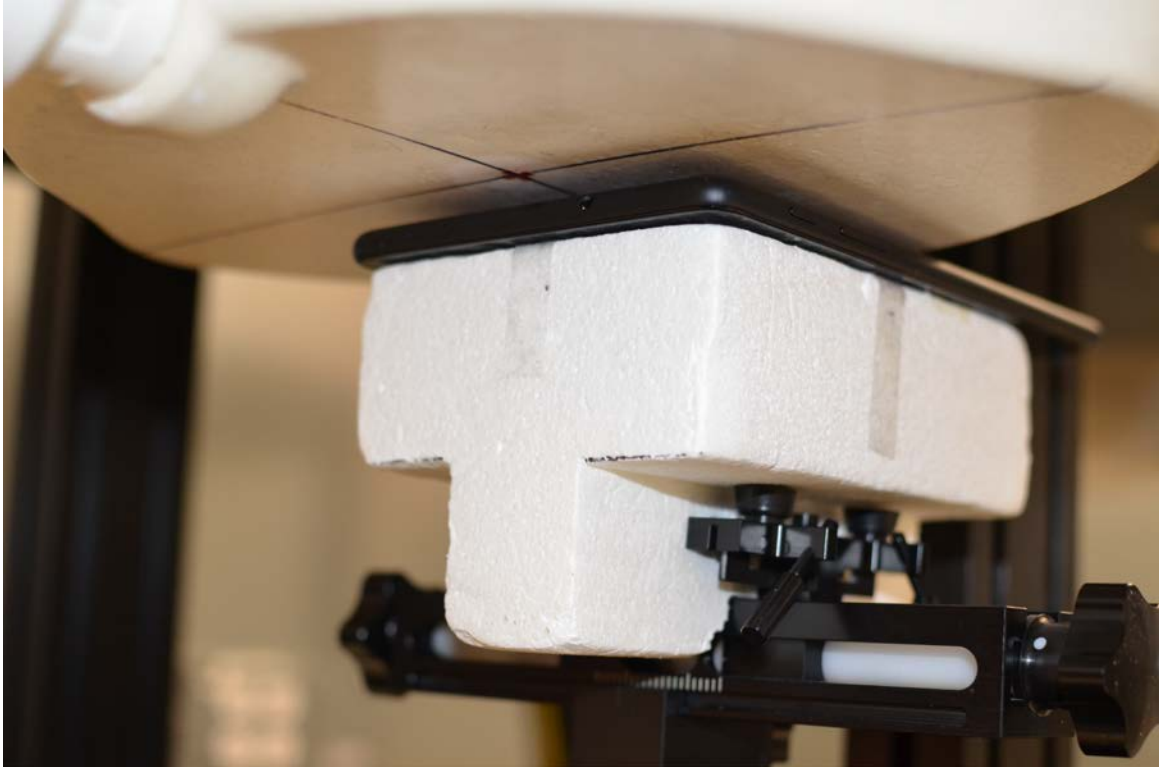
SAR Test Setup Photo 1: Back Side at 0.6 cm
