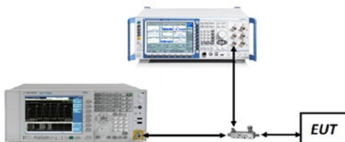
Figure 7-2. Test Instrument & Measurement Setup
