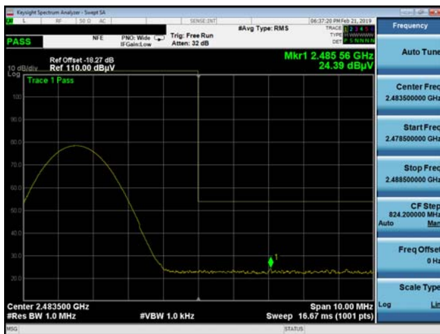
Plot 7-46. Radiated Restricted Upper Band Edge Measurement (Average)
