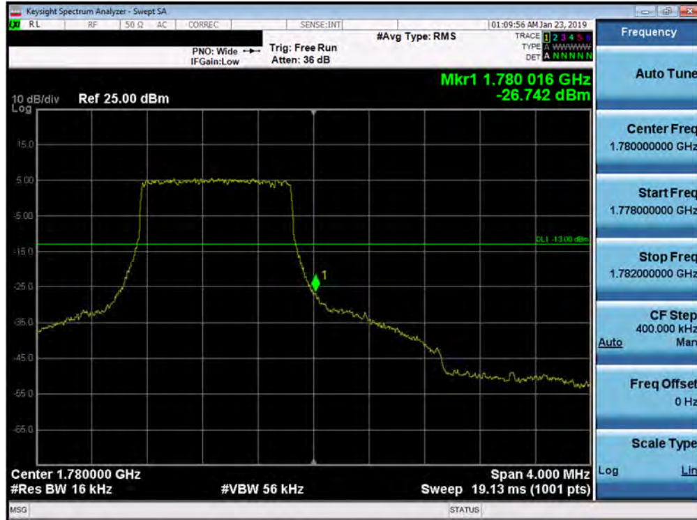
Plot 7-116. Upper Band Edge Plot (Band 66 - 1.4MHz QPSK - Full RB Configuration)
