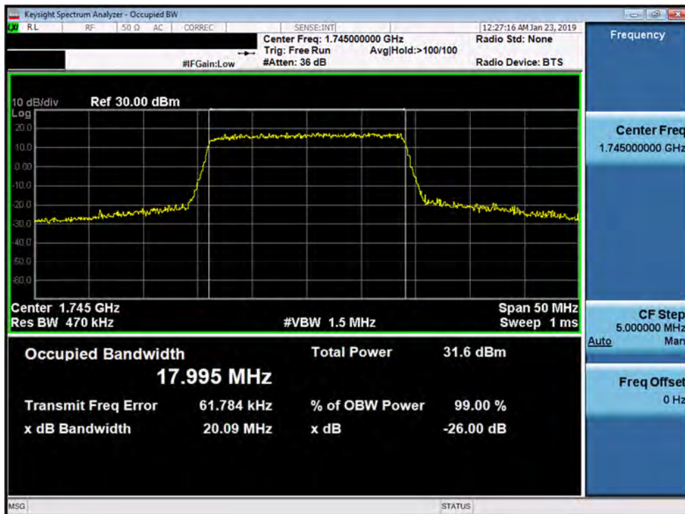
Plot 7-28. Occupied Bandwidth Plot (Band 66/4 - 20.0MHz 16-QAM - Full RB Configuration)
