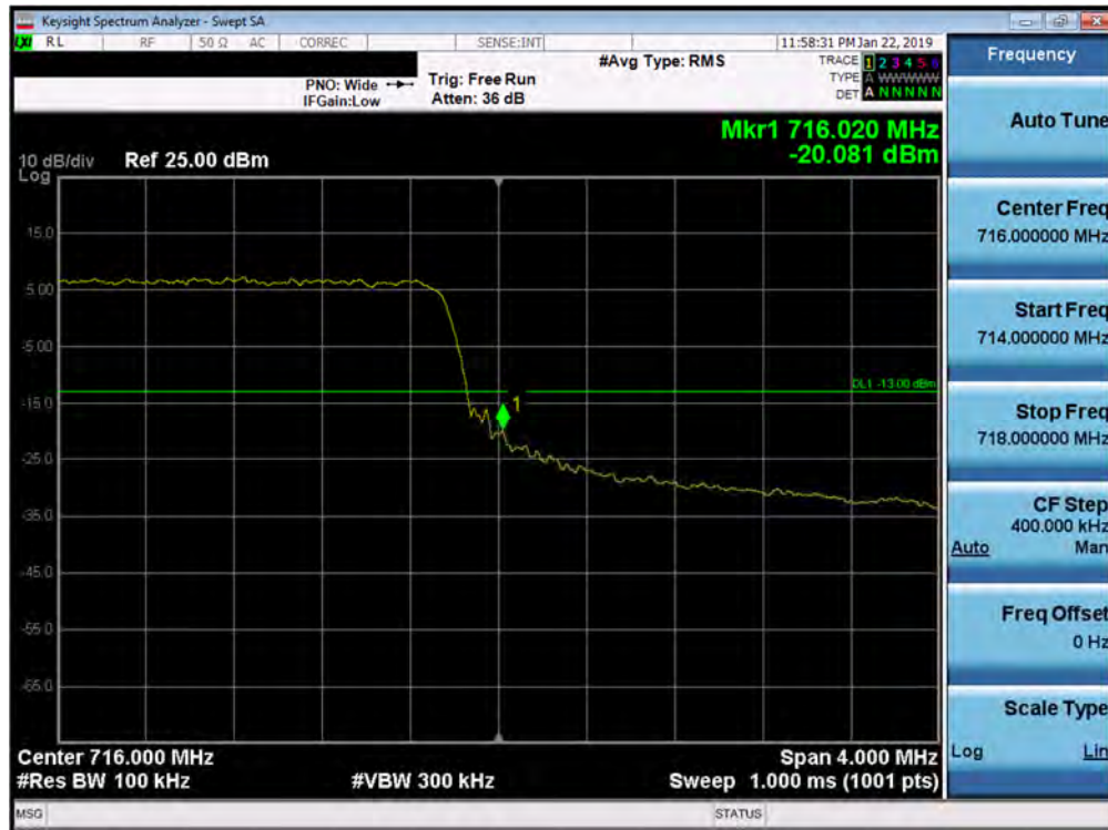
Plot 7-100. Upper Band Edge Plot (Band 12/17 - 5.0MHz QPSK - Full RB Configuration)
