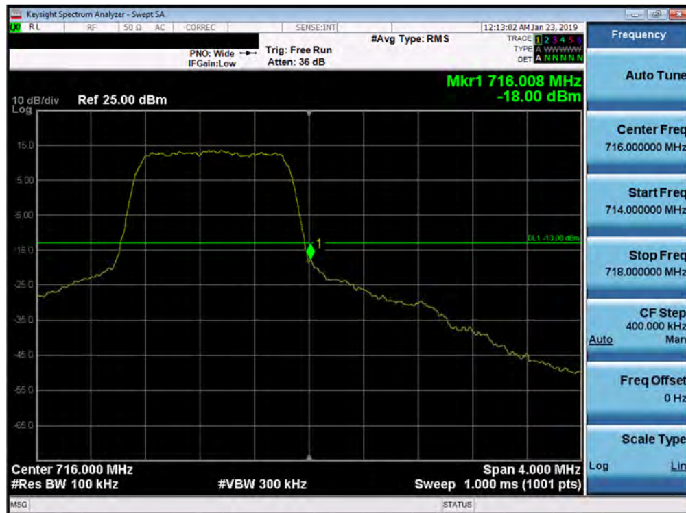
Plot 7-95. Upper Band Edge Plot (Band 12 - 1.4MHz QPSK - Full RB Configuration)
