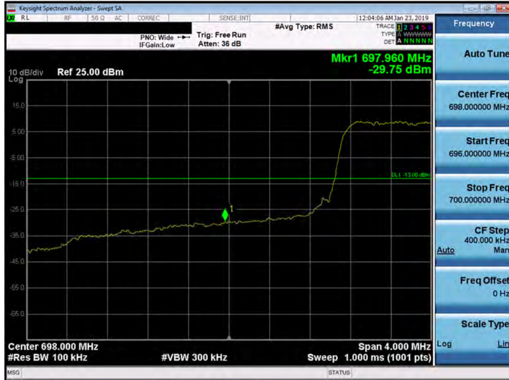
Plot 7-96. Lower Band Edge Plot (Band 12 - 3.0MHz QPSK - Full RB Configuration)
