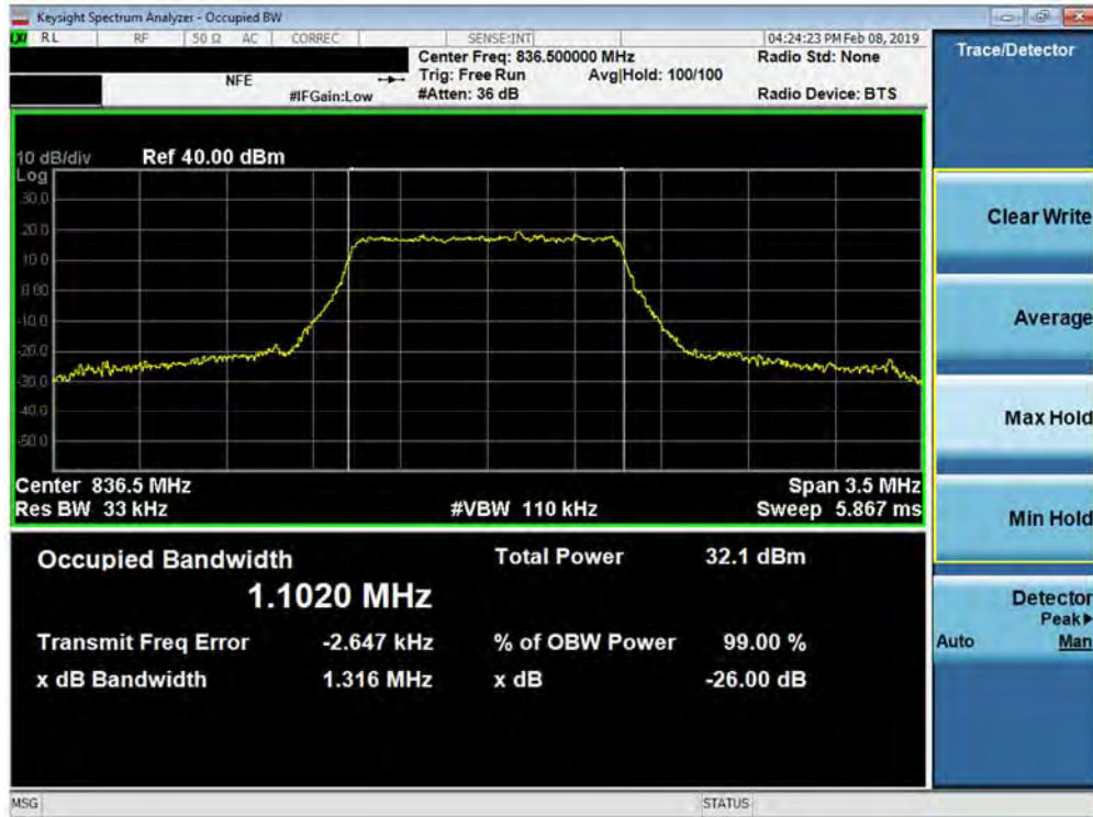
Plot 7-9. Occupied Bandwidth Plot (Band 5 - 1.4MHz QPSK - Full RB Configuration)
