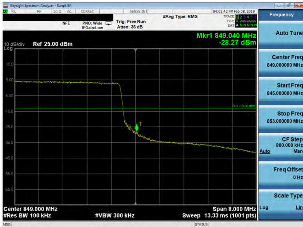
Plot 7-111. Upper Band Edge Plot (Band 5 - 10.0MHz QPSK - Full RB Configuration)
