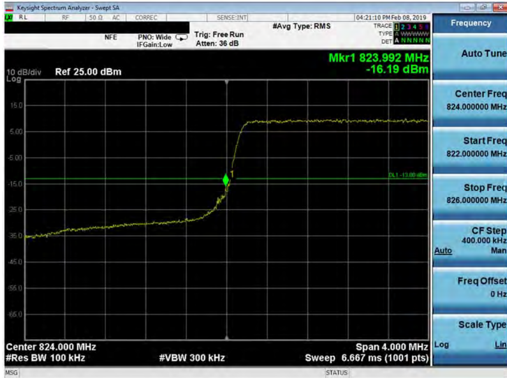
Plot 7-106. Lower Band Edge Plot (Band 5 - 3.0MHz QPSK - Full RB Configuration)
