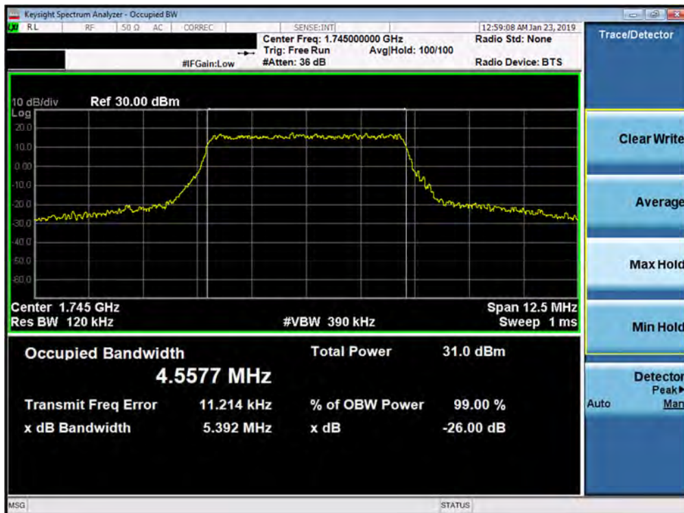
Plot 7-22. Occupied Bandwidth Plot (Band 66/4 - 5.0MHz 16-QAM - Full RB Configuration)
