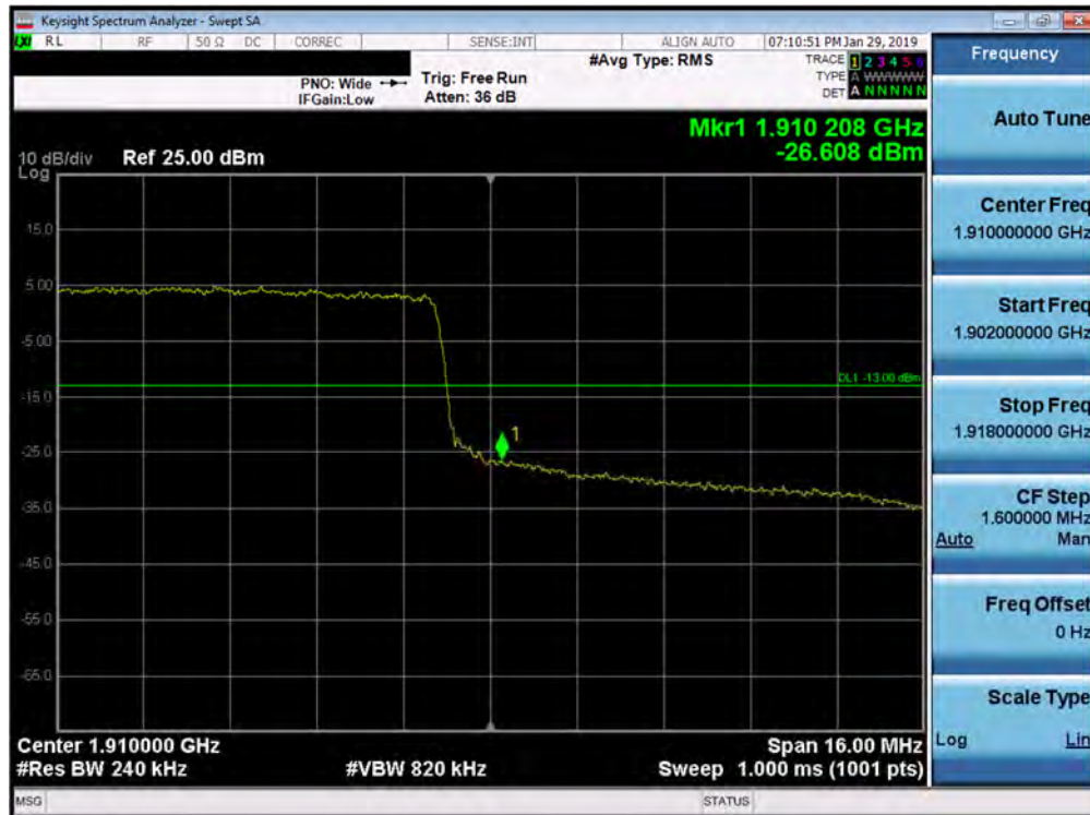
Plot 7-170. Upper Band Edge Plot (Band 2 - 20.0MHz QPSK - Full RB Configuration)
