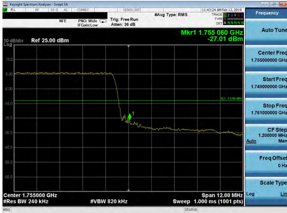
Plot 7-138. Upper Band Edge Plot (Band 4 - 15.0MHz QPSK - Full RB Configuration)
