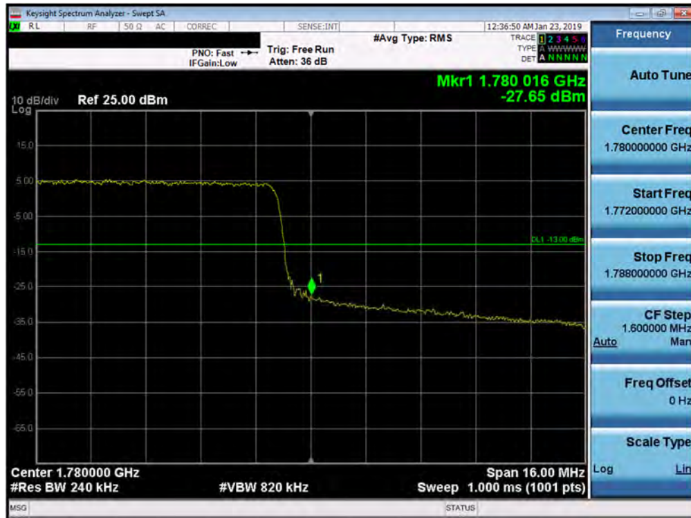
Plot 7-146. Upper Band Edge Plot (Band 66 - 20.0MHz QPSK - Full RB Configuration)
