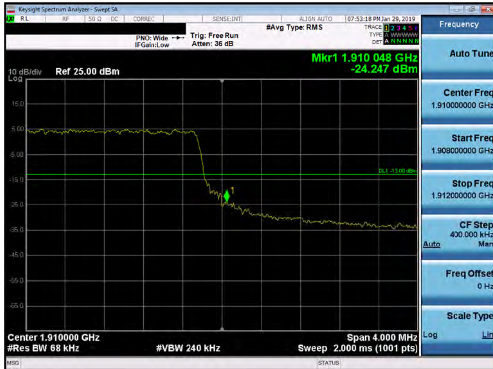
Plot 7-158. Upper Band Edge Plot (Band 2 - 5.0MHz QPSK - Full RB Configuration)
