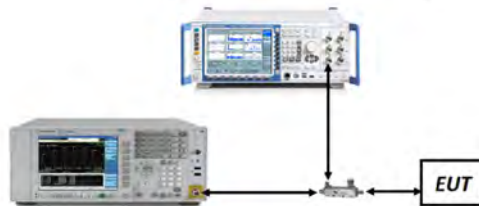
Figure 7-4. Test Instrument & Measurement Setup
