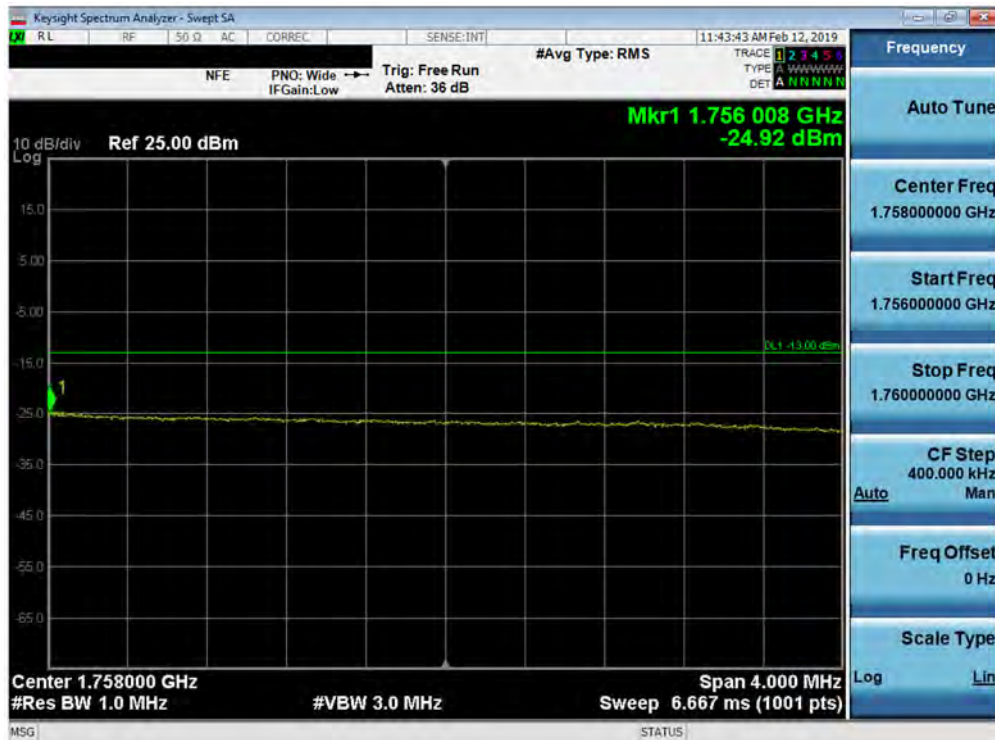
Plot 7-139. Upper Extended Band Edge Plot (Band 4 - 15.0MHz QPSK - Full RB Configuration)
