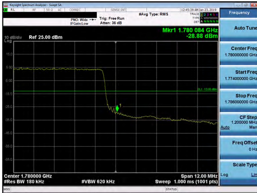
Plot 7-140. Upper Band Edge Plot (Band 66 - 15.0MHz QPSK - Full RB Configuration)
