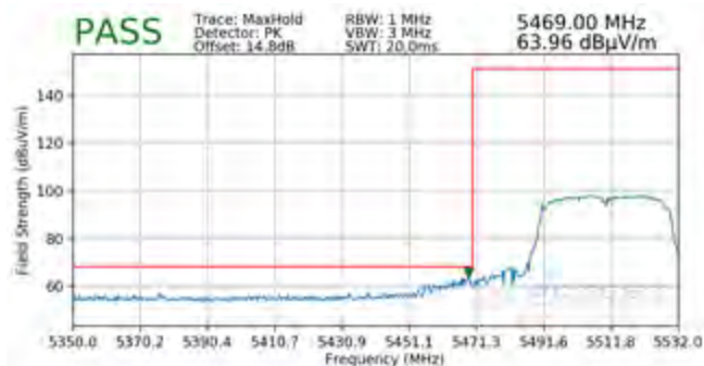
Plot 7-96. Radiated Lower Band Edge Plot SISO ANT1 (Peak – UNII Band 2C)
