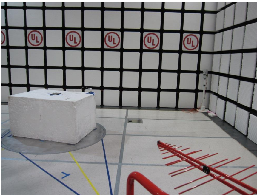
RADIATED FRONT PHOTO (BELOW 1 GHz)
