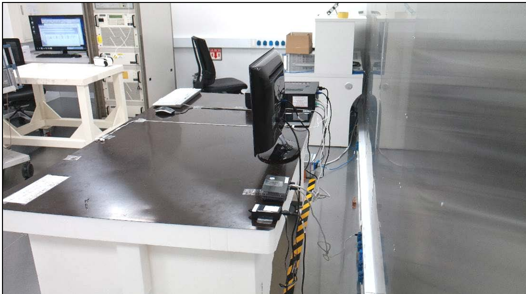
[ Conducted Disturbance – Rear ]
