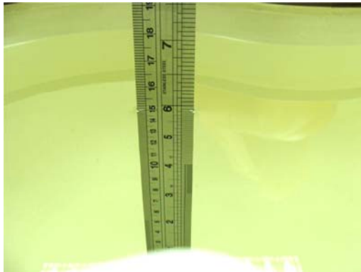
Photo of Liquid Height for Head SAR
