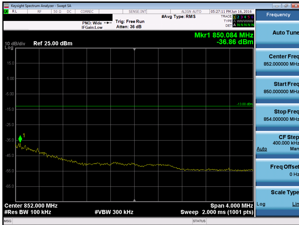
Plot 7-21. Upper Extended Band Edge Plot (Band 5 – 1.4MHz QPSK – RB Size 6)
