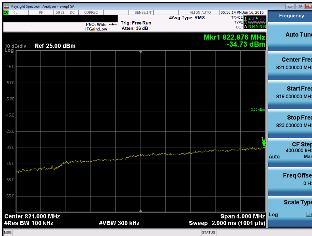
Plot 7-27. Lower Extended Band Edge Plot (Band 5 - 5.0MHz QPSK - RB Size 25)
